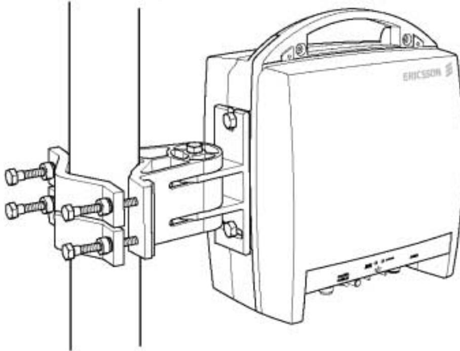
**Figure 3-3. The assembled radio unit and antenna.**
