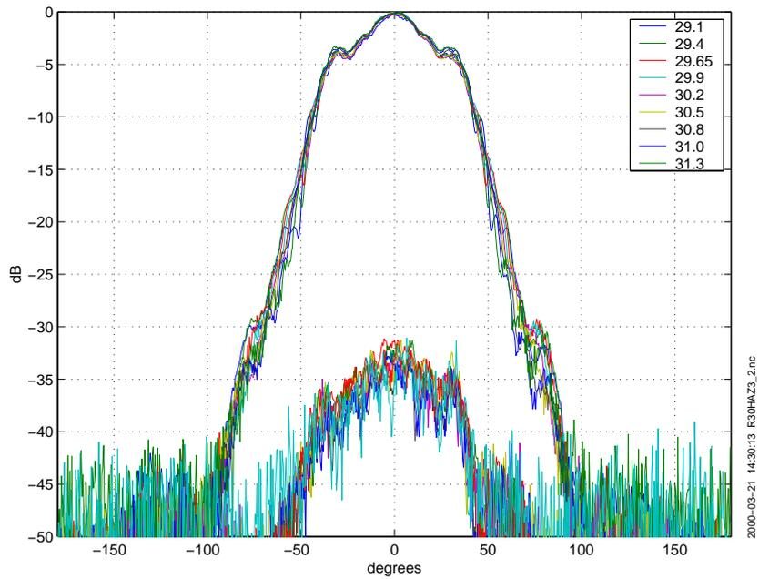
**Figure 7** Radiation patterns in azimuth for antenna #3.
