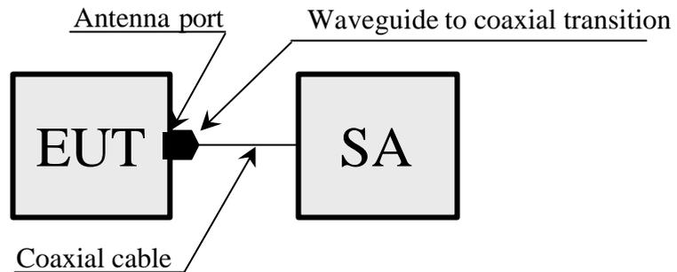
**EUT = Equipment Under Test**
