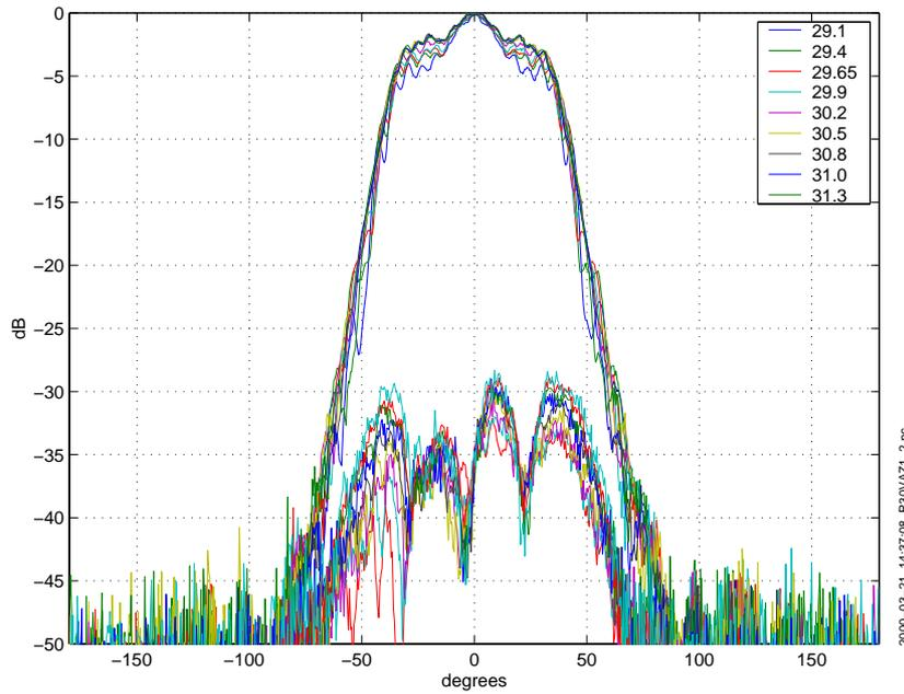
**Figure 11** Radiation patterns in azimuth for A23000HUJA.
