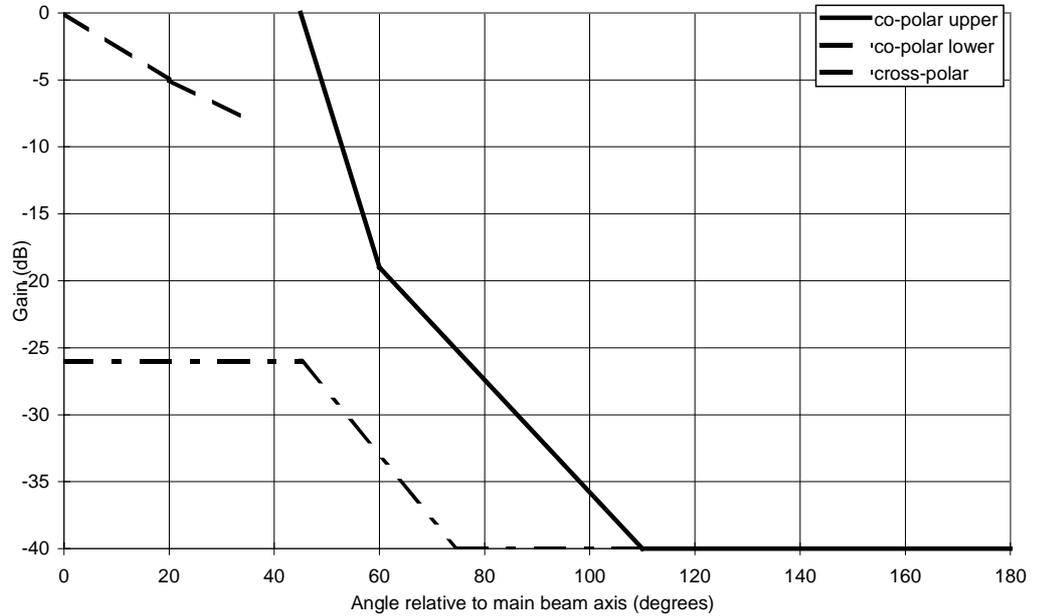
**Figure 2.1** Guaranteed azimuth radiation pattern envelope (RPE), Radio node antenna 30 GHz.
