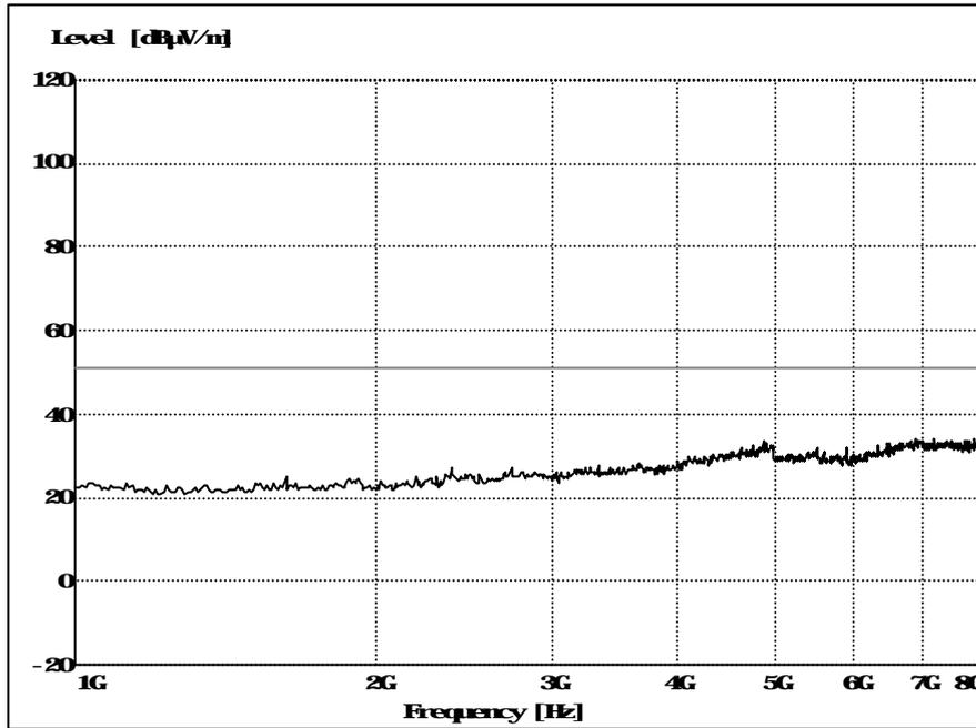
Figure 5. Radiated emission 1 – 8 GHz, Background.
