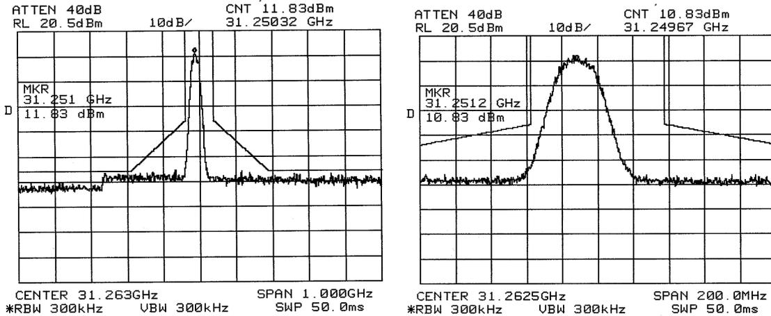
**Figure 8-9. 31.251GHz - 1<sup>st</sup> channel lower band end measurement.**
