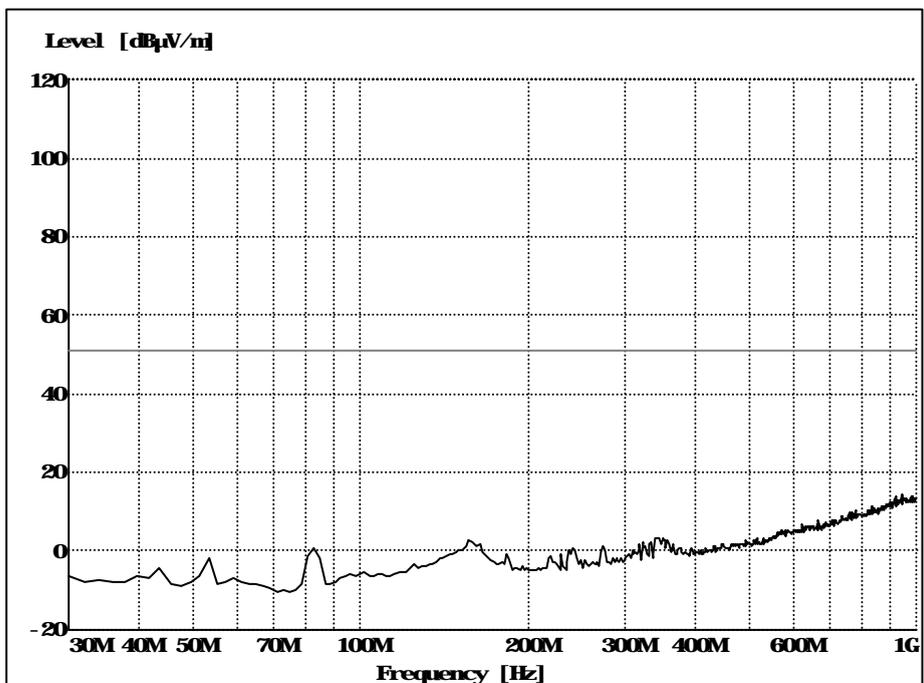
Figure 10. Radiated emission 30 M – 1 GHz, Background measurement.
