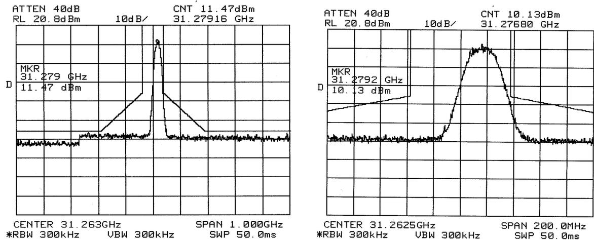
**Figure 10-11 31.279GHz - 2<sup>nd</sup> channel higher band end measurement.**
