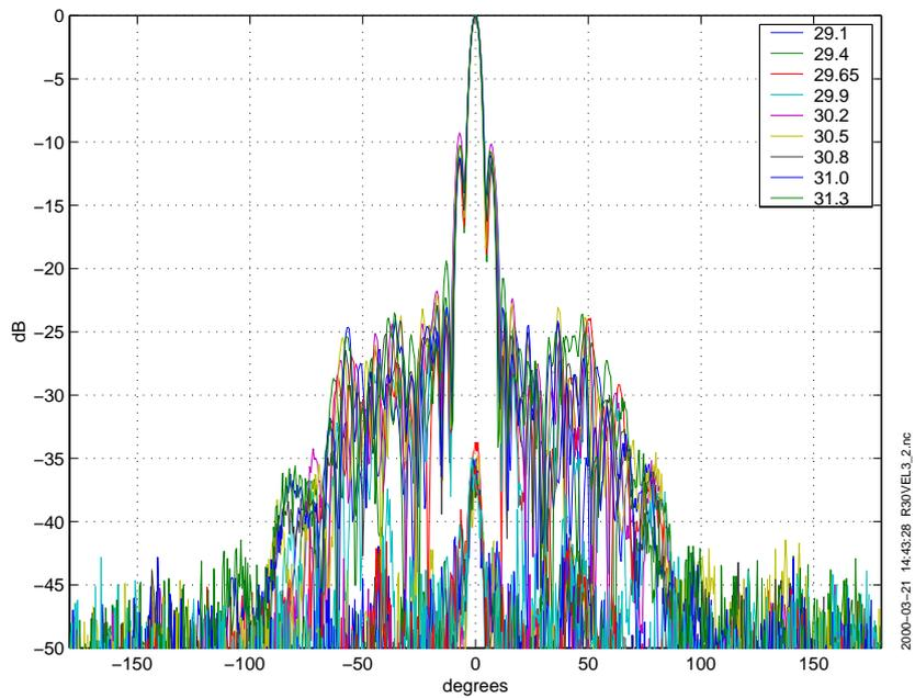
**Figure 16** Radiation patterns in elevation for A23000HUJ9.
