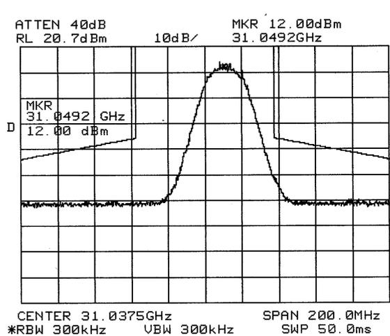
**Figure 5-6. 31.049GHz - 2<sup>nd</sup> channel higher band end measurement.**
