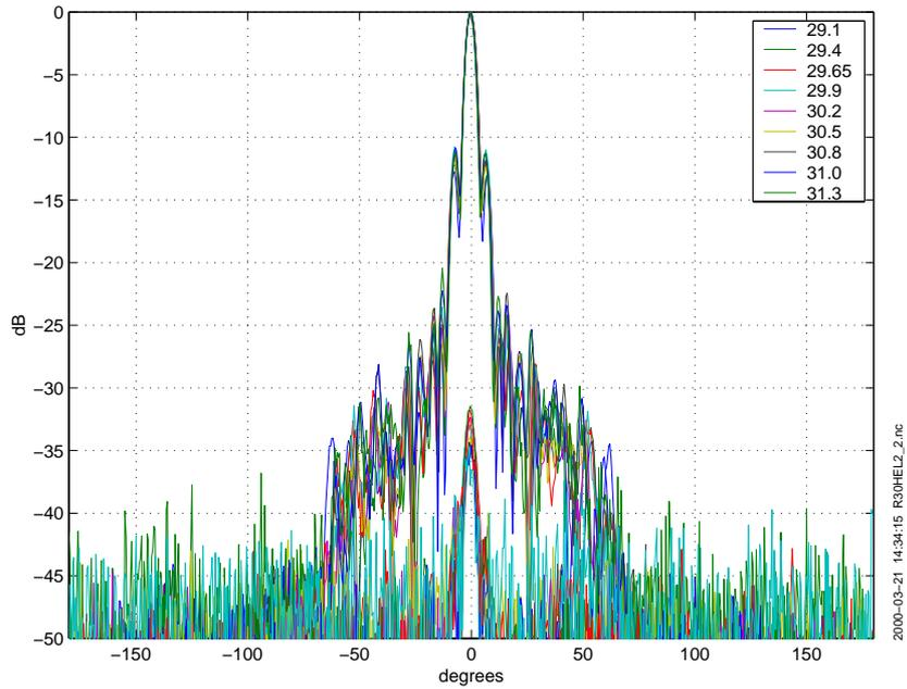
**Figure 9** Radiation patterns in elevation for antenna #2.
