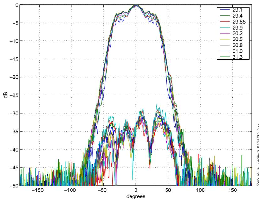
**Figure 12** Radiation patterns in azimuth for A23000HUJB.
