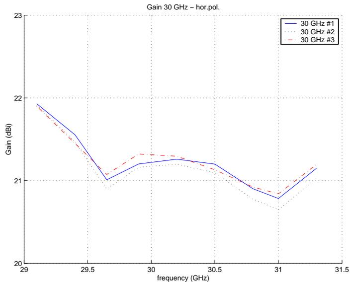
**Figure 1** Gain measurements for some horizontally polarized antennas.
