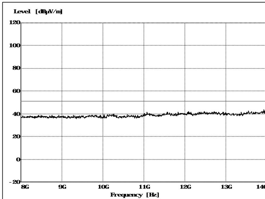
Figure 5. Radiated emission 8 – 14 GHz, Background.
