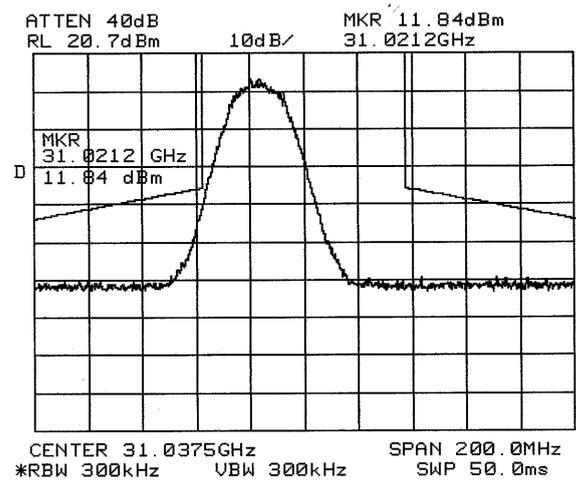
**Figure 4-5. 31.021GHz - 1<sup>st</sup> channel lower band end measurement.**
