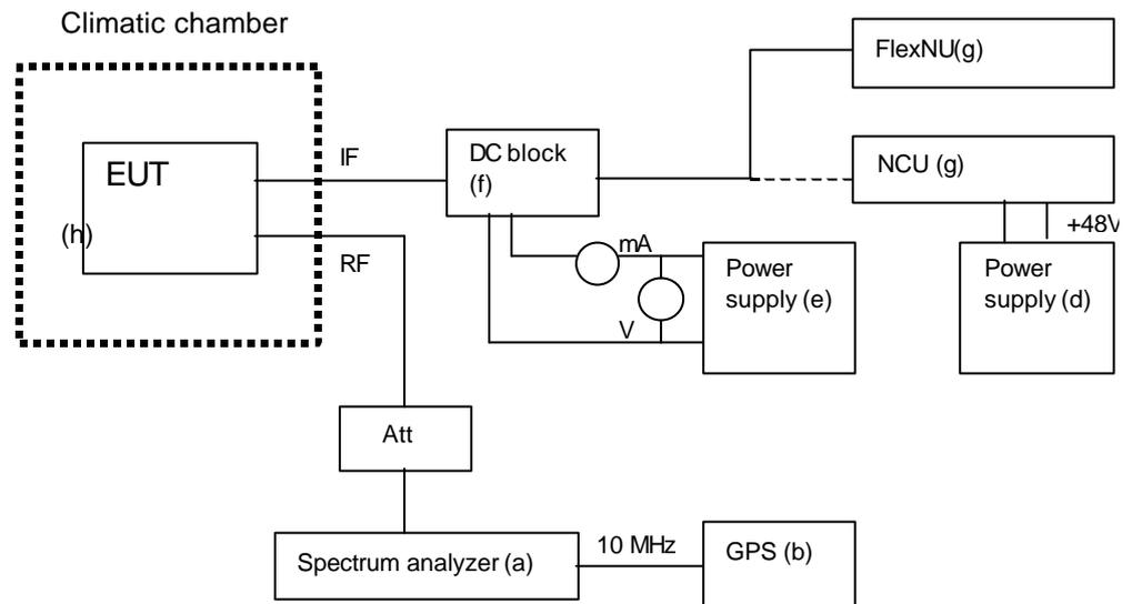
**Figure 1 – Sketch of measurement set-up**
