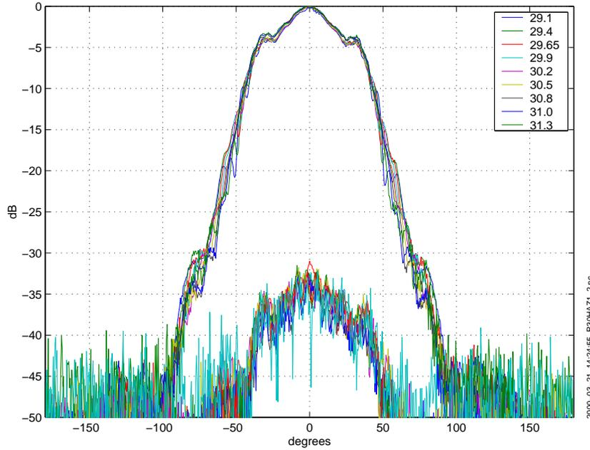
**Figure 5** Radiation pattern in azimuth for antenna #1.
