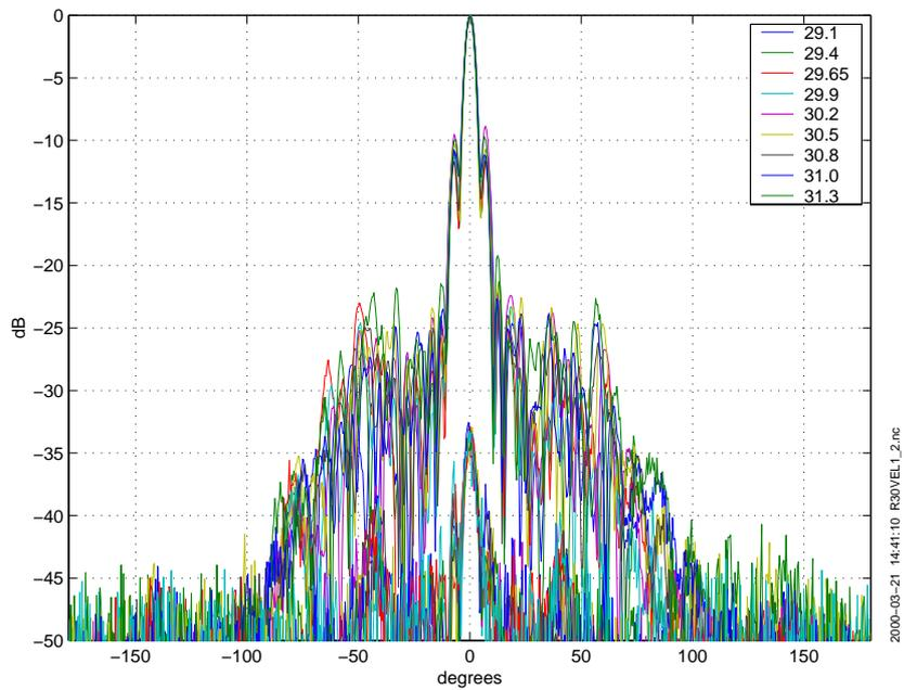
**Figure 14** Radiation patterns in elevation for A23000HUJA.
