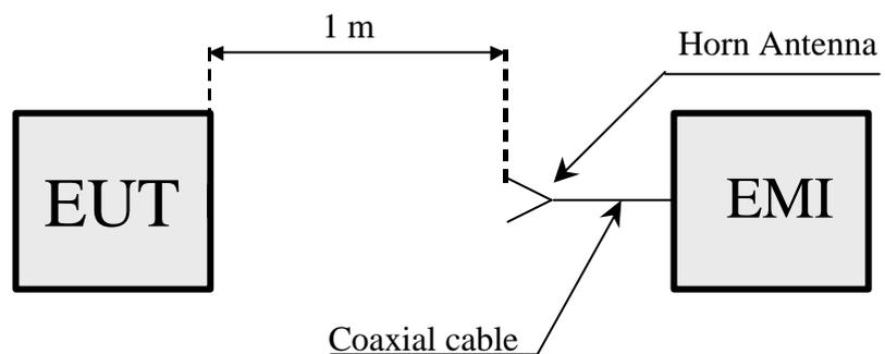
**EUT = Equipment Under Test**
