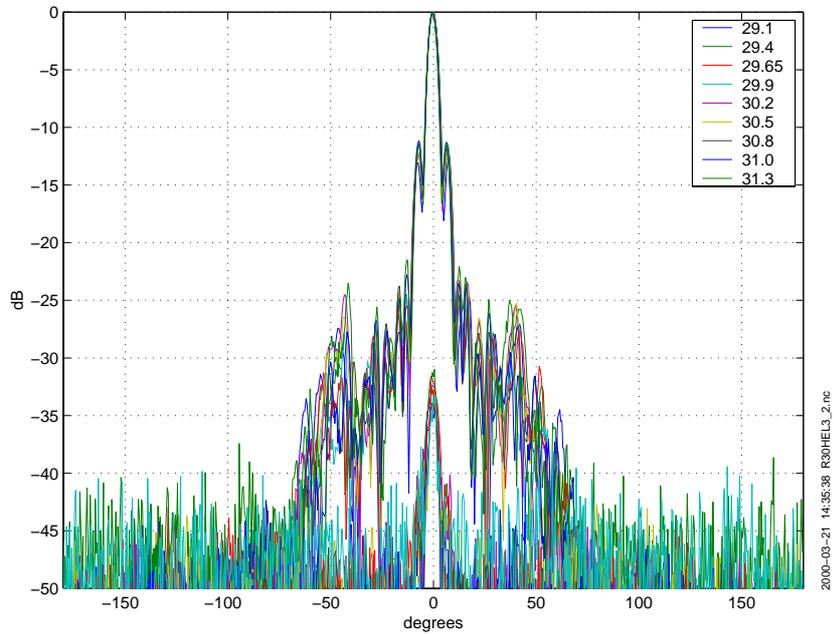
**Figure 10** Radiation patterns in elevation for antenna #3.
