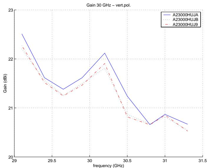
**Figure 2** Gain measurements for some vertically polarized antennas.
