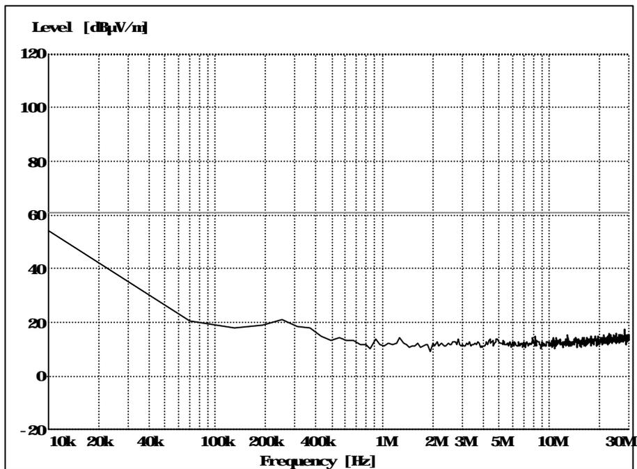
Figure 9. Radiated emission 10 k– 30 MHz, Background.
