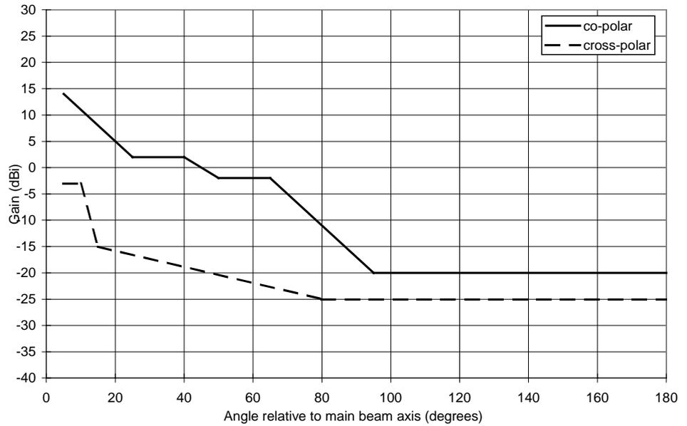
**Figure 2.1** Guaranteed radiation pattern envelope (RPE), 0.2 m compact 30 GHz, high performance.
