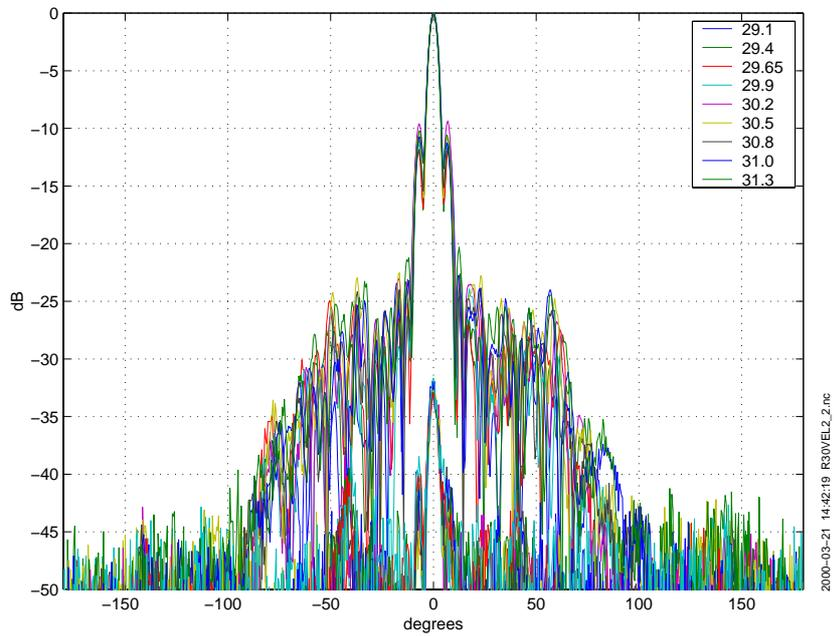
**Figure 15** Radiation patterns in elevation for A23000HUJB.
