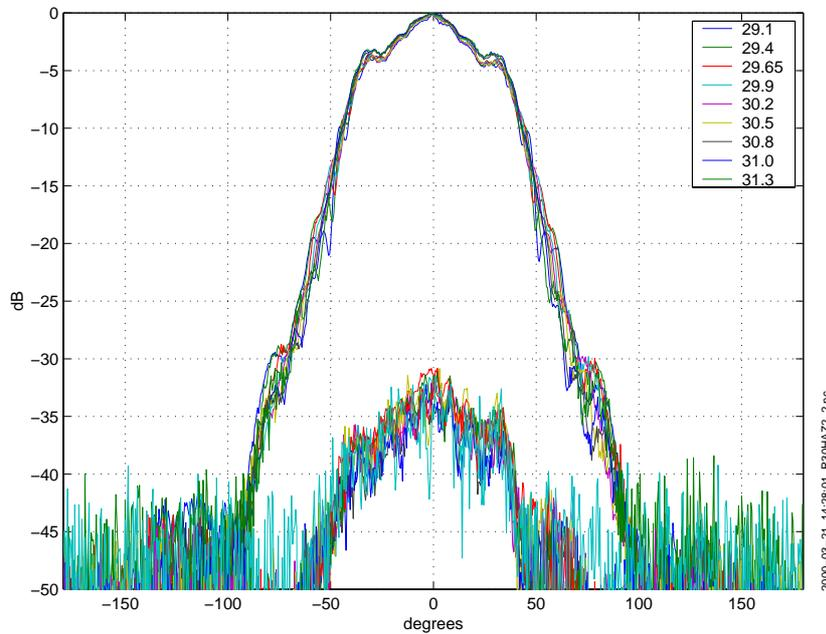
**Figure 6** Radiation pattern in azimuth for antenna #2.
