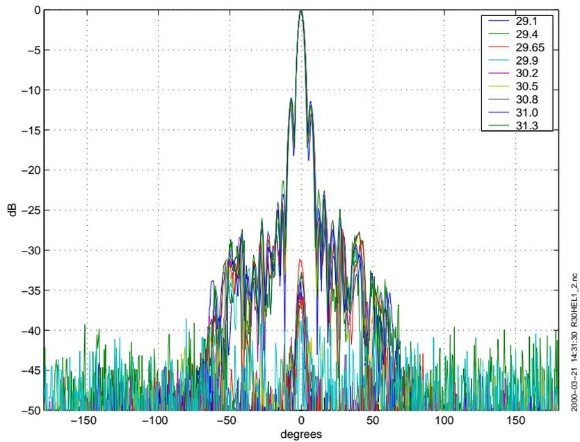
**Figure 8** Radiation patterns in elevation for antenna #1.
