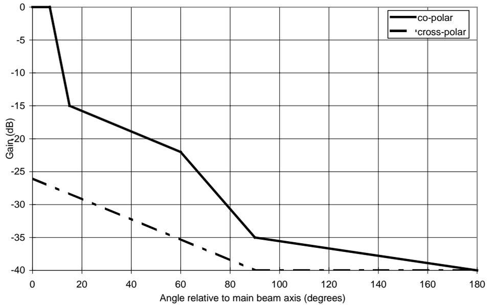
**Figure 2.2** Guaranteed elevation radiation pattern envelope (RPE), Radio node antenna 30 GHz.
