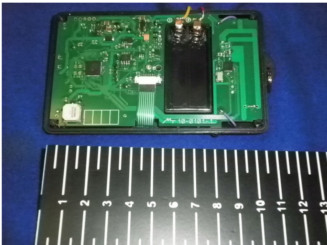
Photograph shows the main NRT302 PCB with the RFID reader / writer module removed.
