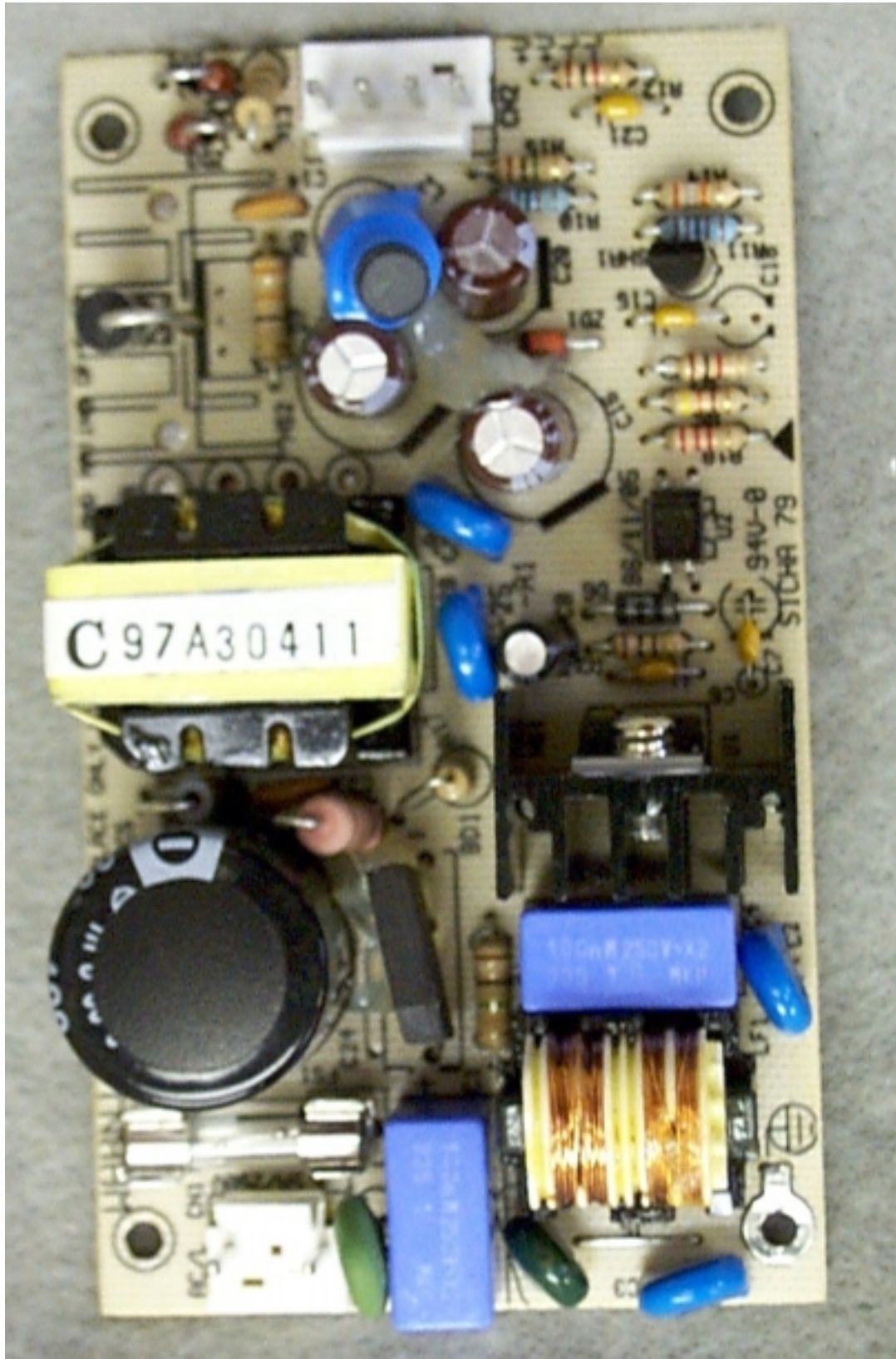
Photo 6. EUT, Top View of Power Supply
