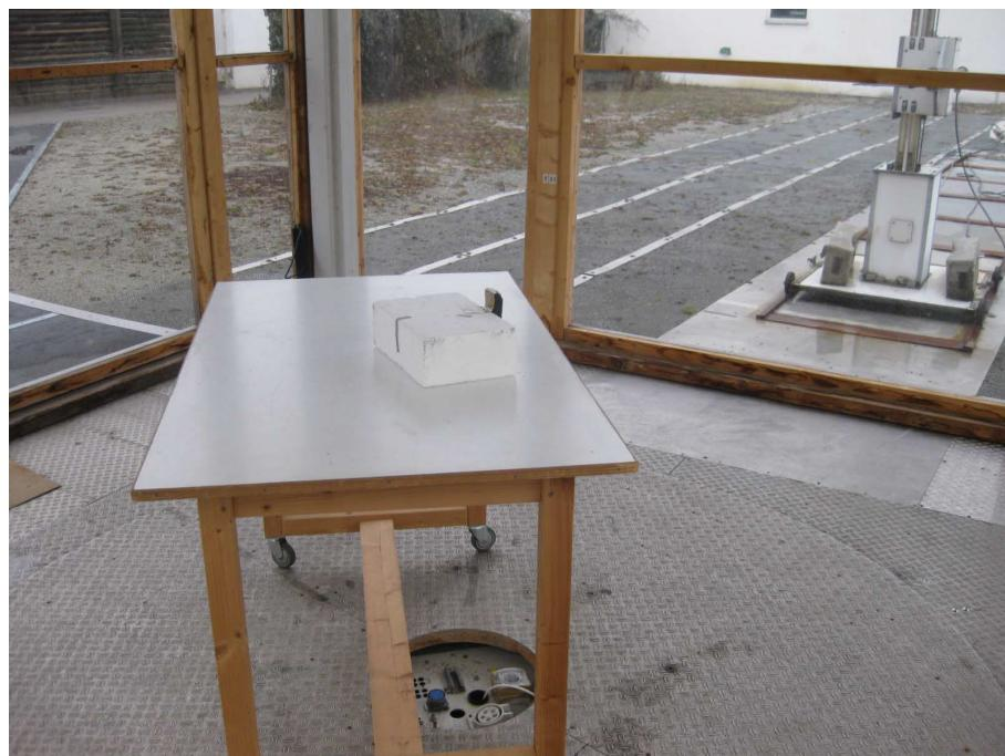
**Test setup for radiated emission measurement
