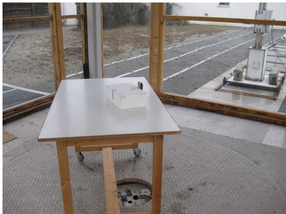
**Test setup for radiated emission measurement
