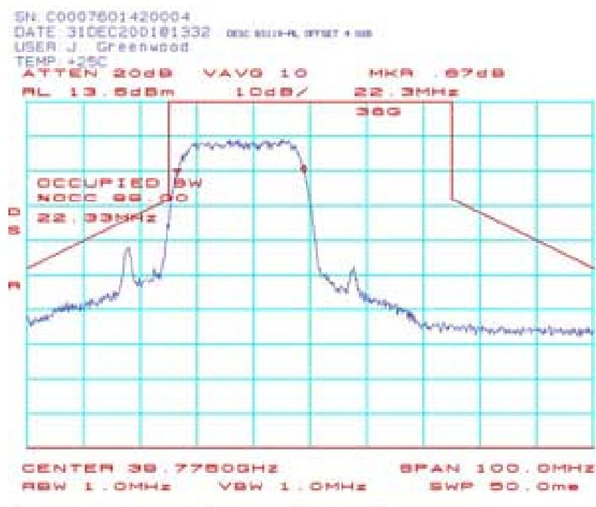
**BS136: Occupied Bandwidth (BS-ODU) 39.7875 GHz 16QAM:**
