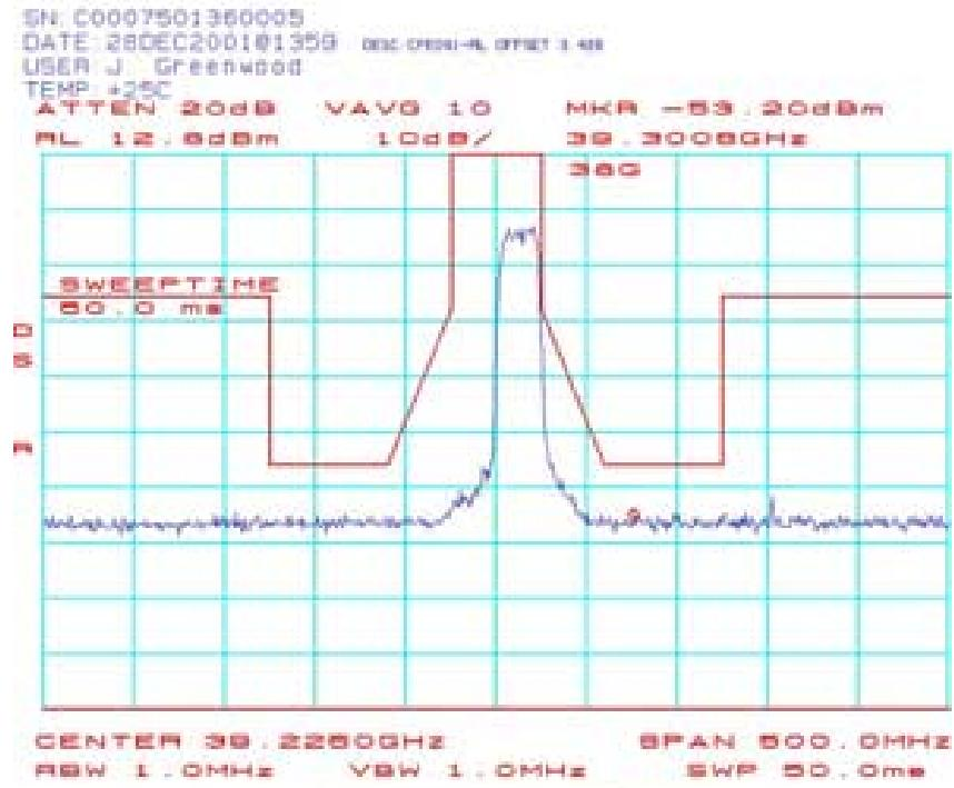
CPE092 Spectrum Mask Plots (CPE-ODU) 39.2375 GHz 64QAM:
