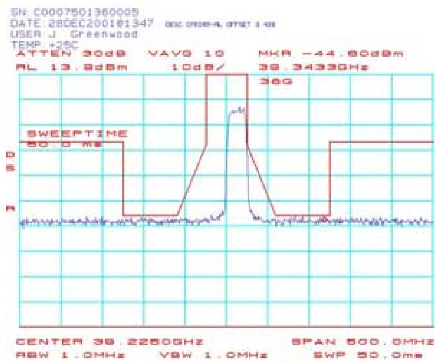
**CPE087 Spectrum Mask Plots (CPE-ODU) 39.2375 GHz 16QAM:**
