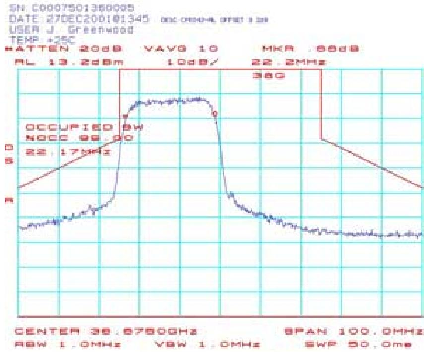
**CPE058: Occupied Bandwidth (CPE-ODU) 38.6875 GHz 16QAM:**
