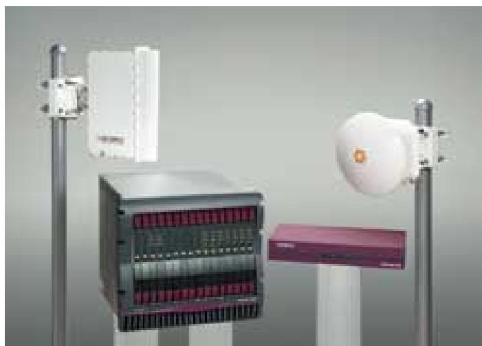
The 16200 Series Base Station Indoor Unit and 320 Series Customer Premises Equipment Indoor Unit operate with a range of outdoor unit transceivers in the range of 10 to 45 GHz. The configuration tested operates in the 38.65 to 39.8GHz frequency band. Both the 16200 Series BS-IDU and the 320 Series CPE-IDU are connected to the 3900 Series ODU transceivers by a single RG-6 coaxial cable and can be separated by up to 1000 feet.
