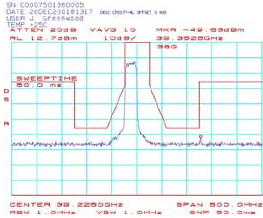
CPE078: Spectrum Mask Plots (CPE-ODU) 39.2125 GHz 64QAM:
