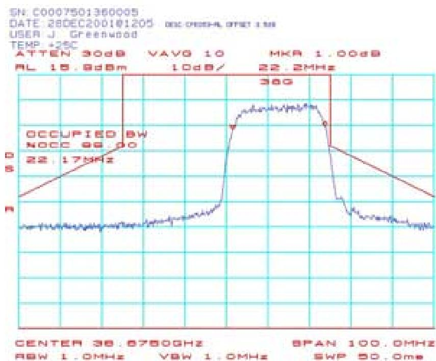
**CPE042: Occupied Bandwidth (CPE-ODU) 38.6625 GHz 16QAM:**
