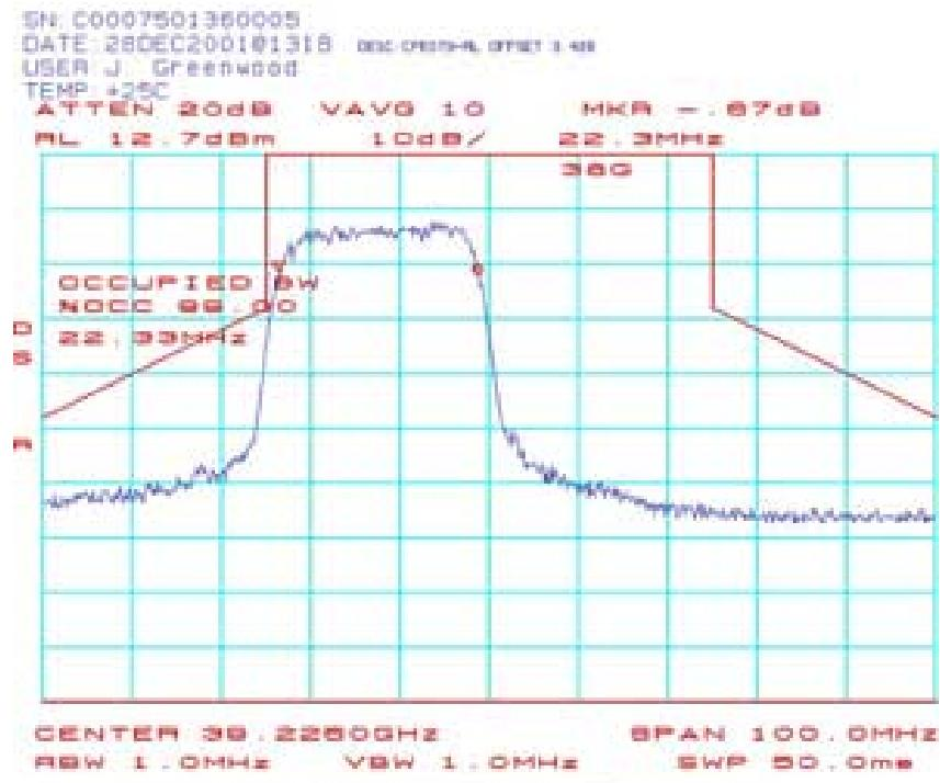
CPE093: Occupied Bandwidth (CPE-ODU) 39.2375 GHz 64QAM:
