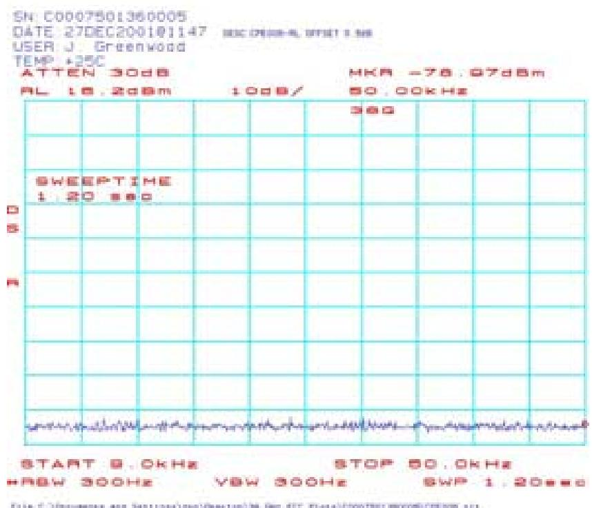
CPE007: Spurious Emission Plots (CPE-ODU) 50 kHz-100 kHz
