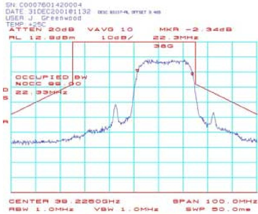
**BS112: Occupied Bandwidth (BS-ODU) 39.7625 GHz QPSK:**
