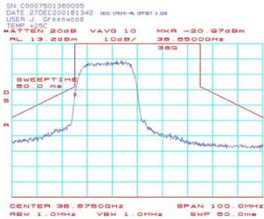
CPE043 Spectrum Mask Plots (CPE-ODU) 38.6625 GHz 16QAM:
