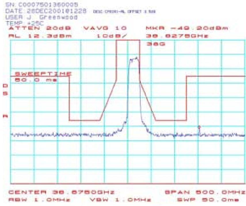
**CPE062 Spectrum Mask Plots (CPE-ODU) 38.6875 GHz 64QAM:**
