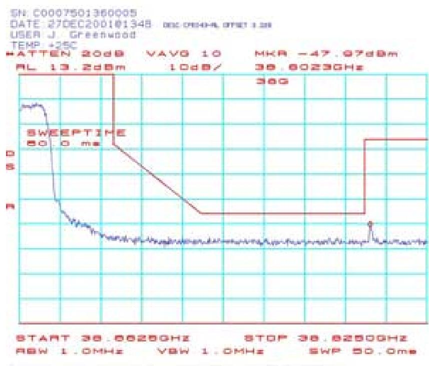
CPE046 Spectrum Mask Plots (CPE-ODU) 38.6625 GHz 64QAM:
