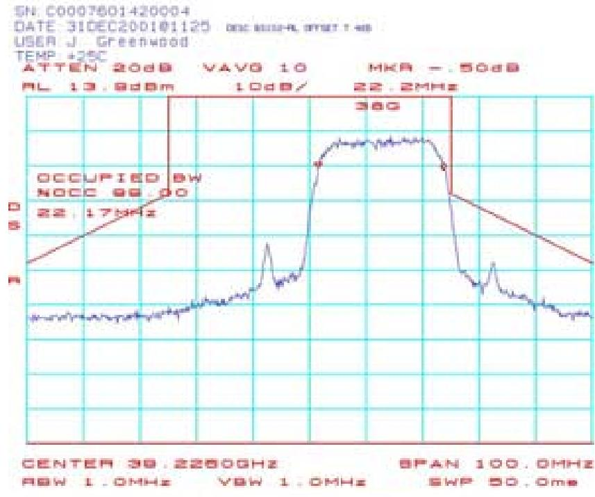
**BS091: Occupied Bandwidth (BS-ODU) 39.2125 GHz 64QAM:**
