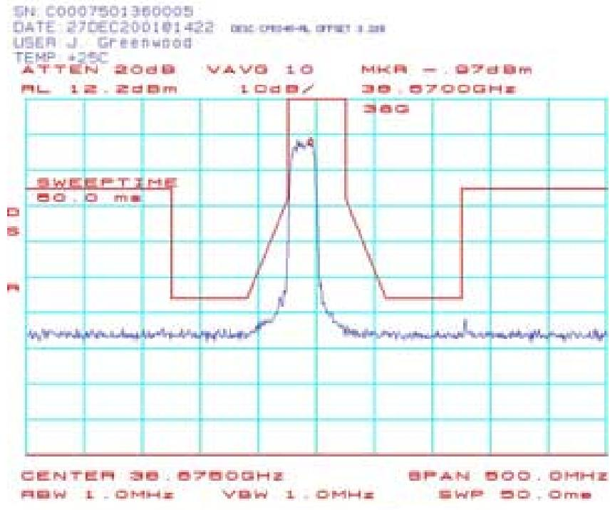
CPE047 Spectrum Mask Plots (CPE-ODU) 38.6625 GHz 64QAM:
