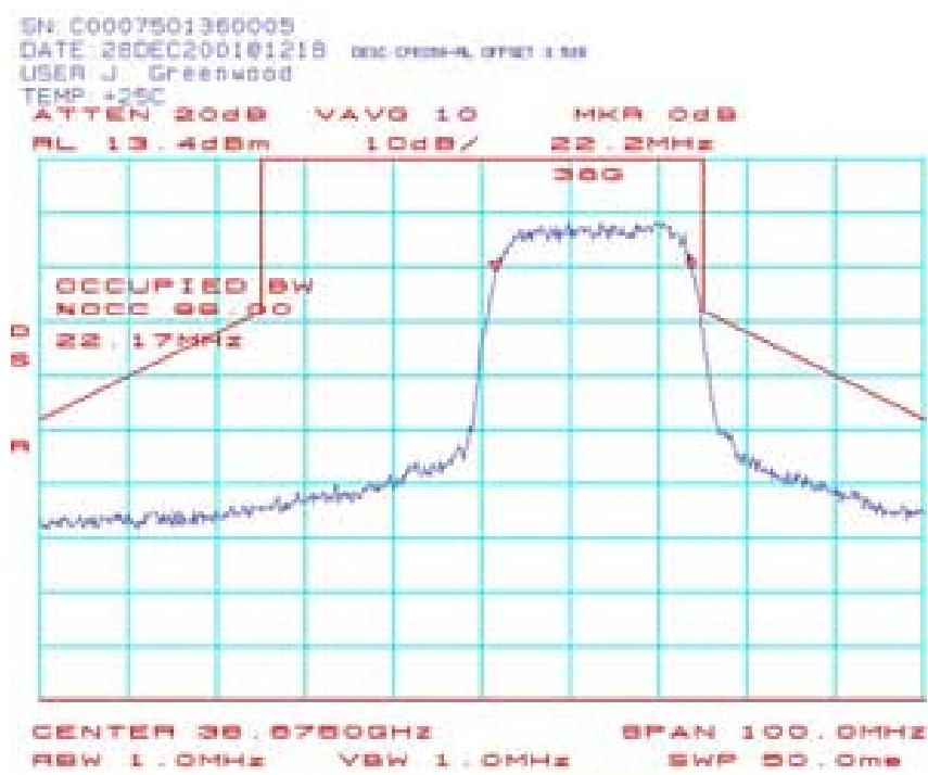
**CPE048: Occupied Bandwidth (CPE-ODU) 38.6625 GHz 64QAM:**
