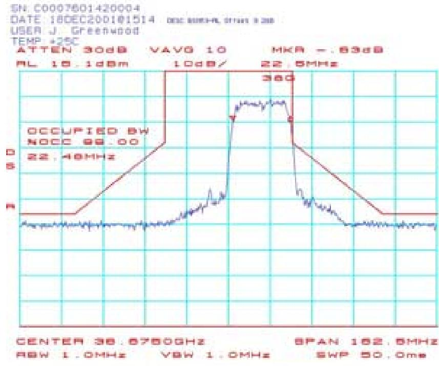
BS053: Occupied Bandwidth (BS-ODU) 38.6625 GHz 16QAM:
