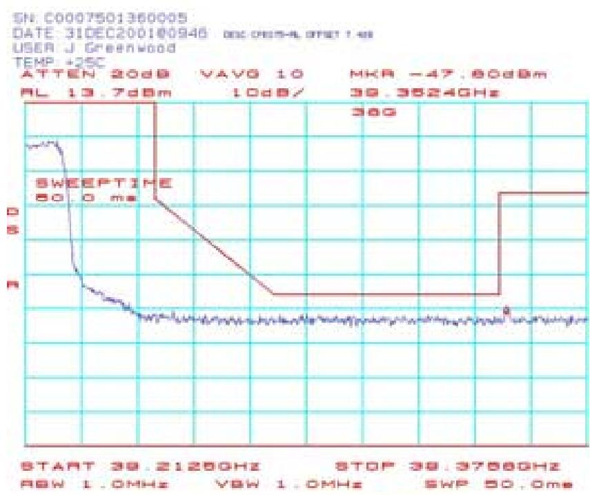
CPE077 Spectrum Mask Plots (CPE-ODU) 39.2125 GHz 64QAM:
