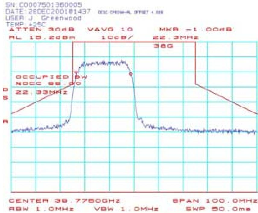
**CPE115: Occupied Bandwidth (CPE-ODU) 39.7875 GHz QPSK:**
