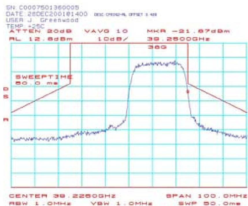
CPE094 Spectrum Mask Plots (CPE-ODU) 39.2375 GHz 64QAM:
