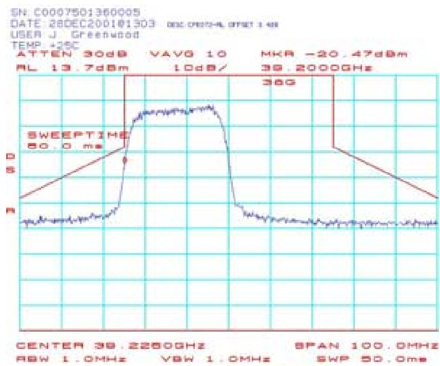
CPE074 Spectrum Mask Plots (CPE-ODU) 39.2125 GHz 16QAM:
