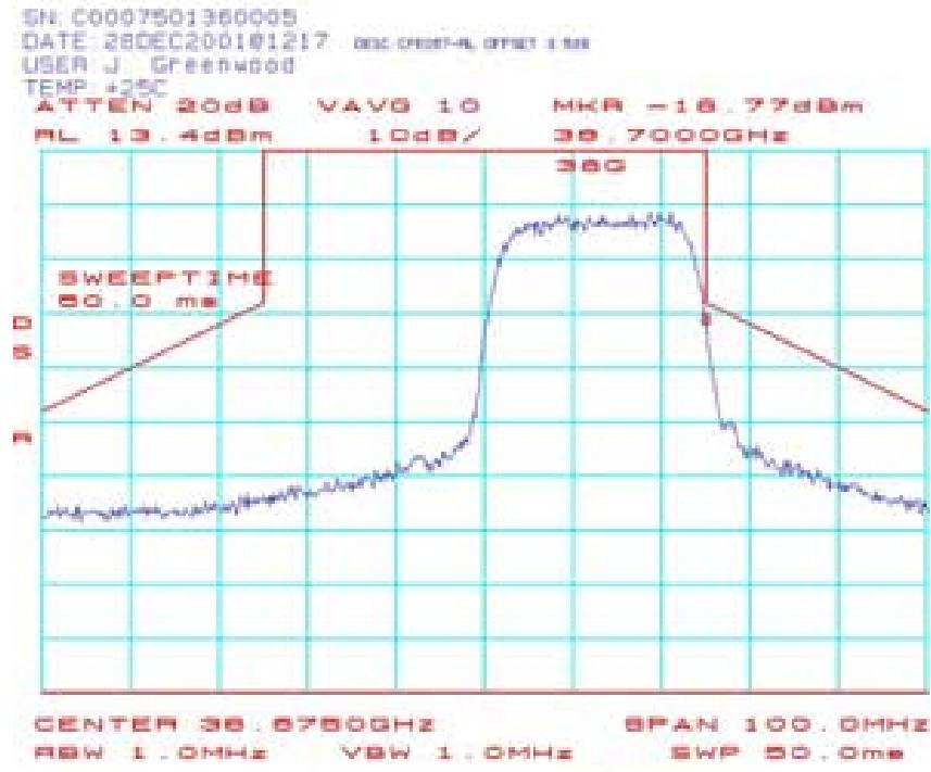
**CPE059 Spectrum Mask Plots (CPE-ODU) 38.6875 GHz 16QAM:**
