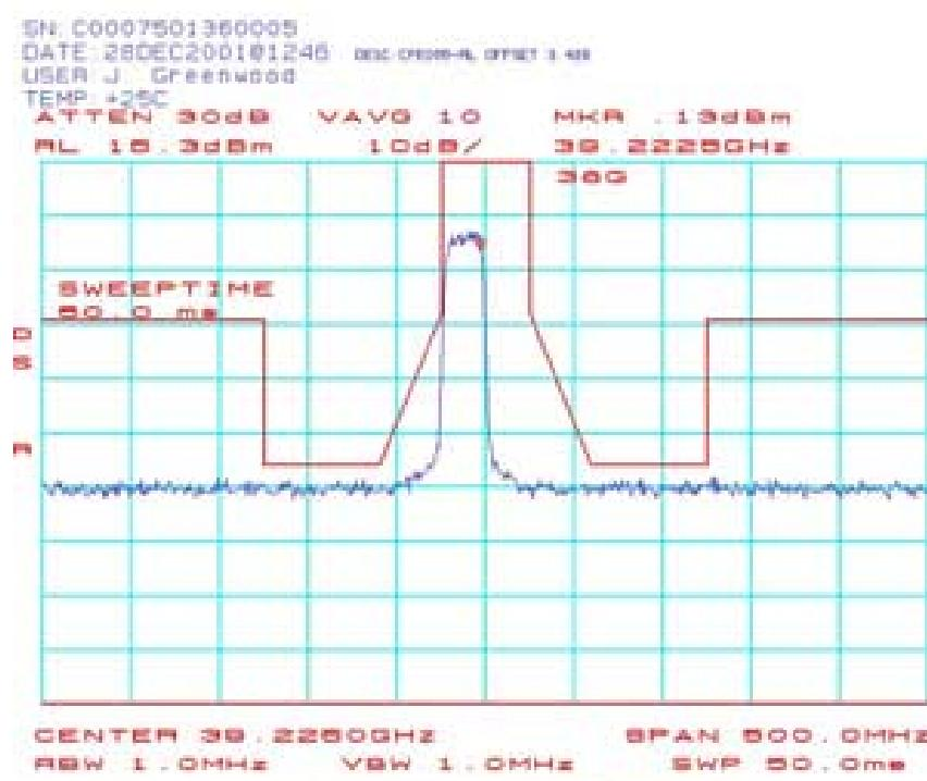
CPE067 Spectrum Mask Plots (CPE-ODU) 39.2125 GHz QPSK:
