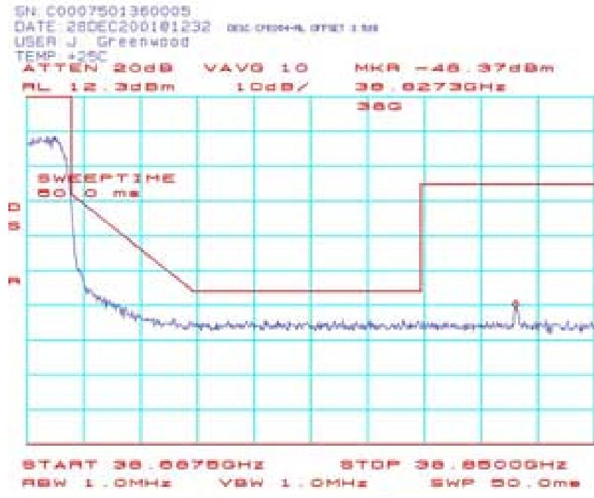
CPE066: Spectrum Mask Plots (CPE-ODU) 39.2125 GHz QPSK:
