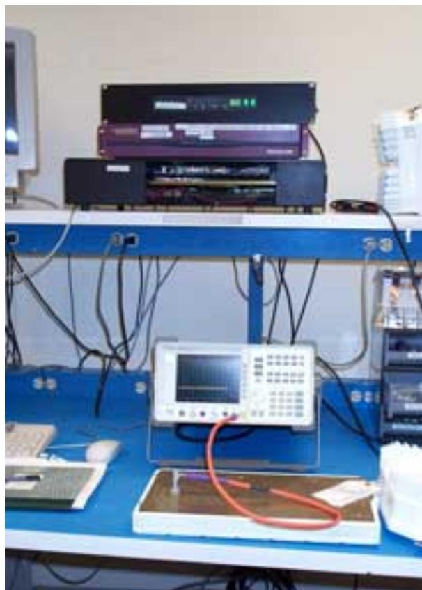
Figure 2 Base Station ODU 9kHz-40GHz Test Set Up
