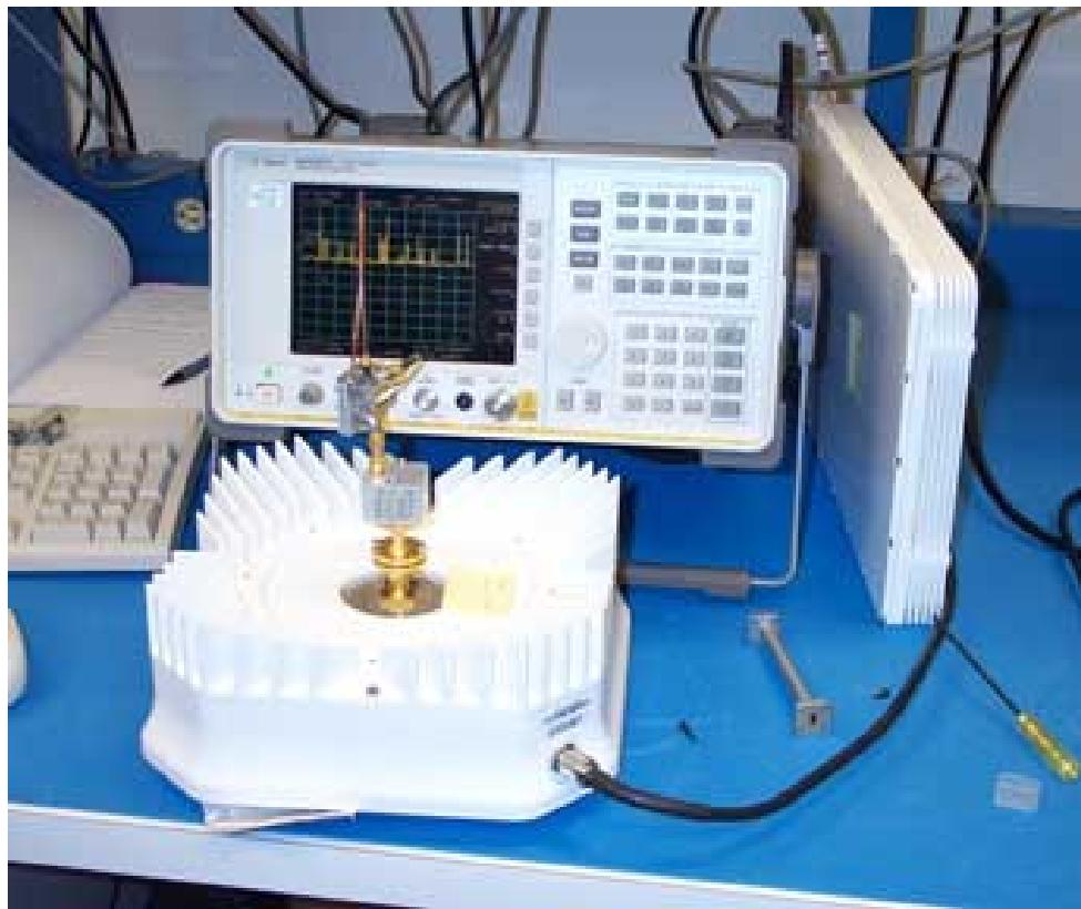
**Figure 6 CPE ODU 40 GHz-200 GHz Test Set Up**
