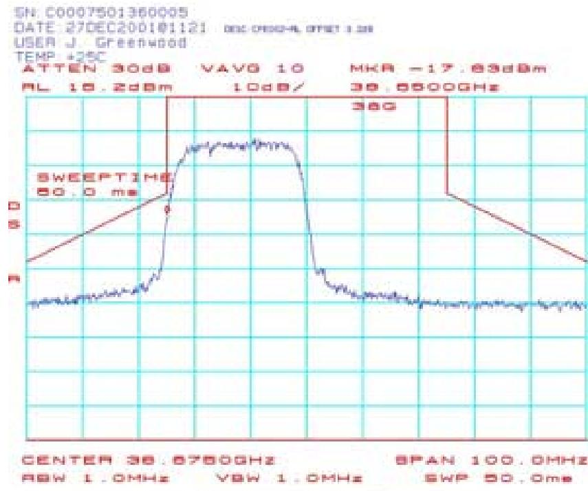
**CPE040: Spectrum Mask Plots (CPE-ODU) 38.6625 GHz 16QAM:**
