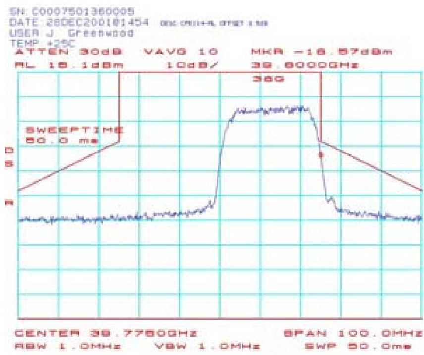
CPE117: Spectrum Mask Plots (CPE-ODU) 39.7875 GHz 16QAM:
