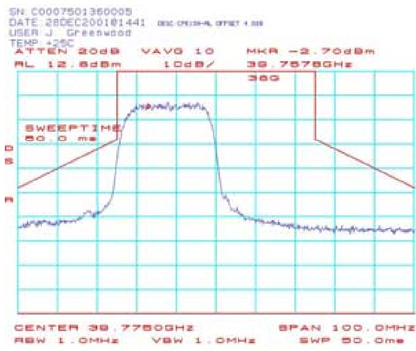
**CPE110: Spectrum Mask Plots (CPE-ODU) 39.3625 GHz 64QAM:**
