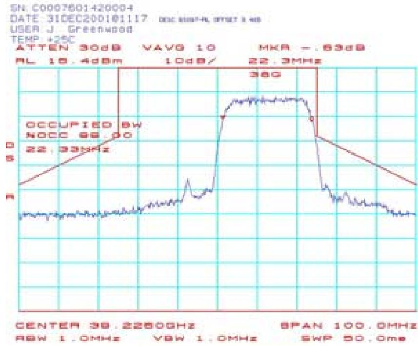
BS084: Occupied Bandwidth (BS-ODU) 39.2125 GHz 16QAM:
