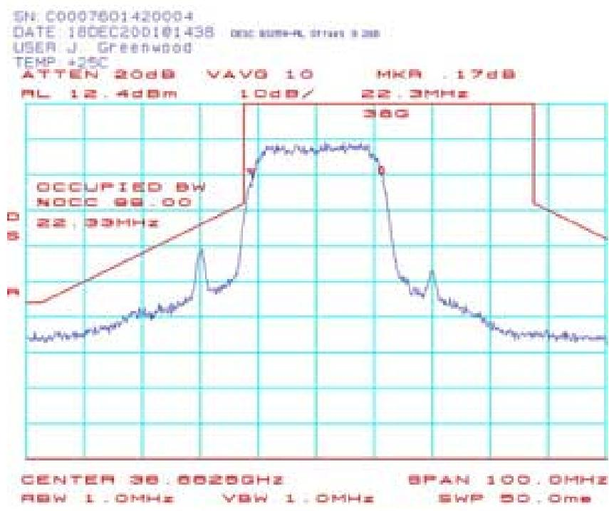
**BS073: Occupied Bandwidth (BS-ODU) 38.6875 GHz 64QAM:**
