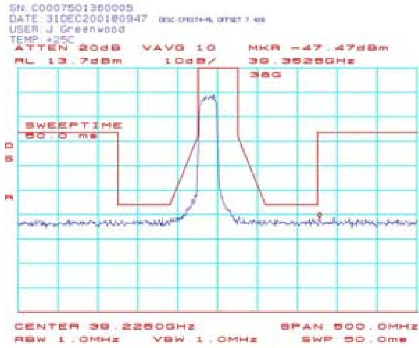
CPE075: Spectrum Mask Plots (CPE-ODU) 39.2125 GHz 16QAM:
