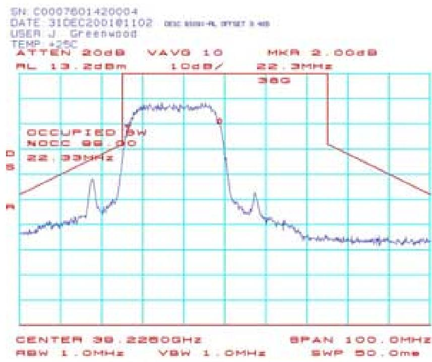
**BS107: Occupied Bandwidth (BS-ODU) 39.2375 GHz 64QAM:**
