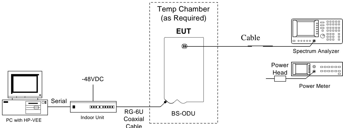
Figure 1 Base Station ODU Test Set Up Drawing
