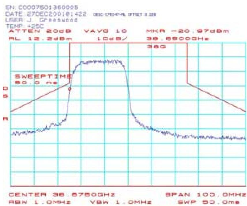
CPE049: Spectrum Mask Plots (CPE-ODU) 38.6625 GHz 64-QAM:
