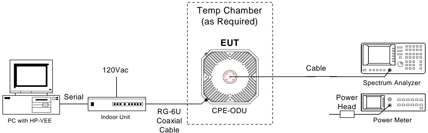
Figure 4 CPE ODU Test Set UP Drawing
