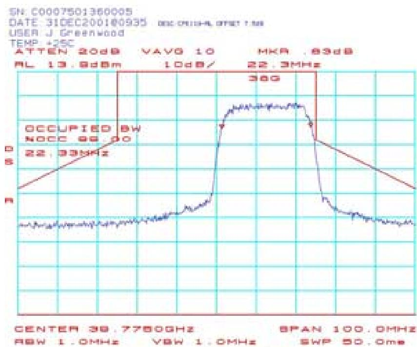
**CPE109: Occupied Bandwidth (CPE-ODU) 39.7625 GHz 64QAM:**
