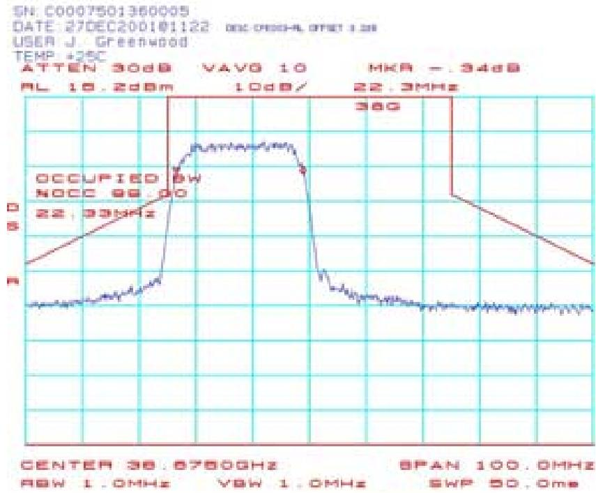
CPE053: Occupied Bandwidth (CPE-ODU) 38.6875 GHz QPSK:
