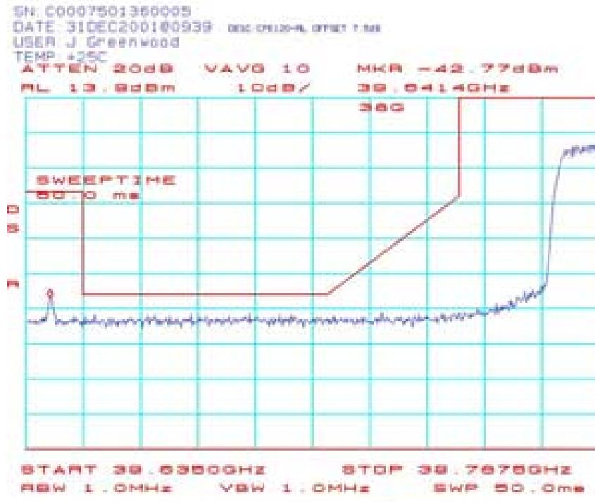
**CPE121: Spectrum Mask Plots (CPE-ODU) 39.7875 GHz 16QAM:**
