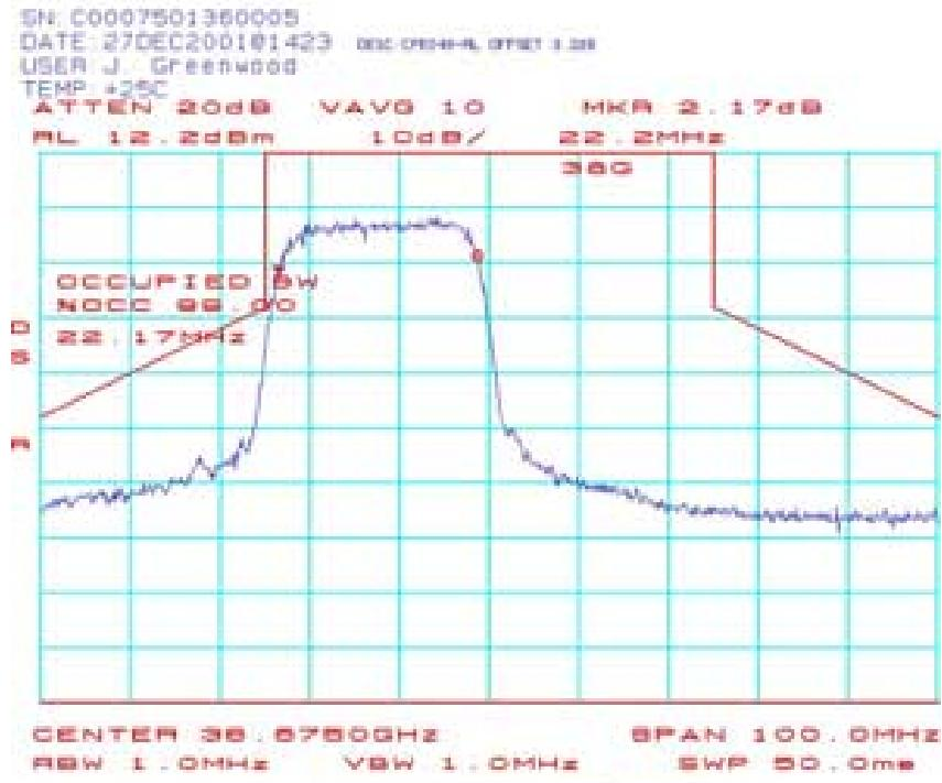
**CPE063: Occupied Bandwidth (CPE-ODU) 38.6875 GHz 64QAM:**
