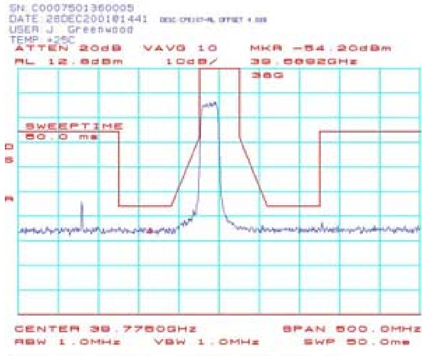
**CPE108: Spectrum Mask Plots (CPE-ODU) 39.3625 GHz 64QAM:**
