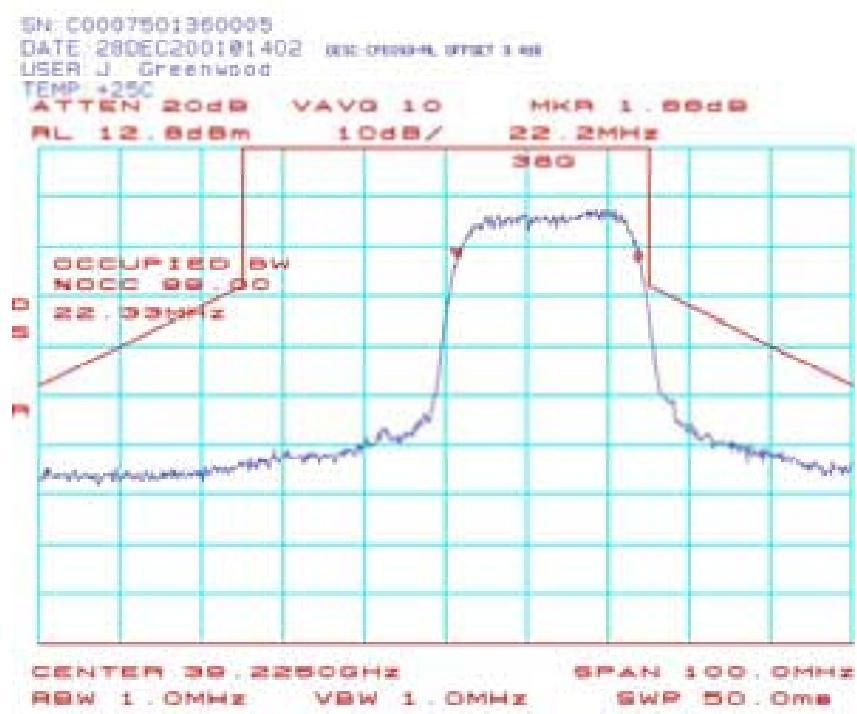
**CPE098: Occupied Bandwidth (CPE-ODU) 39.7625 GHz QPSK:**
