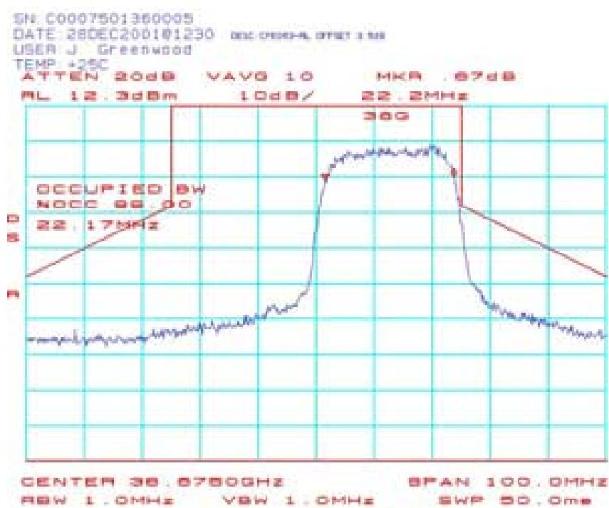
**CPE068: Occupied Bandwidth (CPE-ODU) 39.2125 GHz QPSK:**
