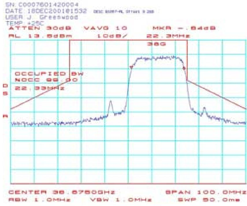
**BS058: Occupied Bandwidth (BS-ODU) 38.6625 GHz 64QAM:**
