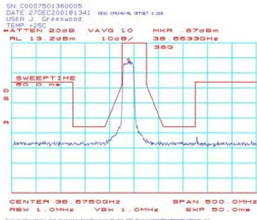
CPE041 Spectrum Mask Plots (CPE-ODU) 38.6625 GHZ 16QAM:
