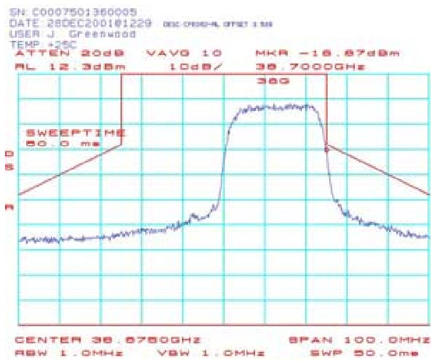
CPE064 Spectrum Mask Plots (CPE-ODU) 38.6875 GHz 64QAM:
