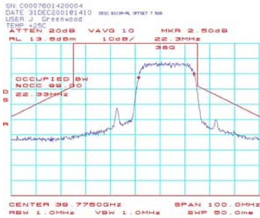
**BS124: Occupied Bandwidth (BS-ODU) 39.7625 GHz 64QAM:**
