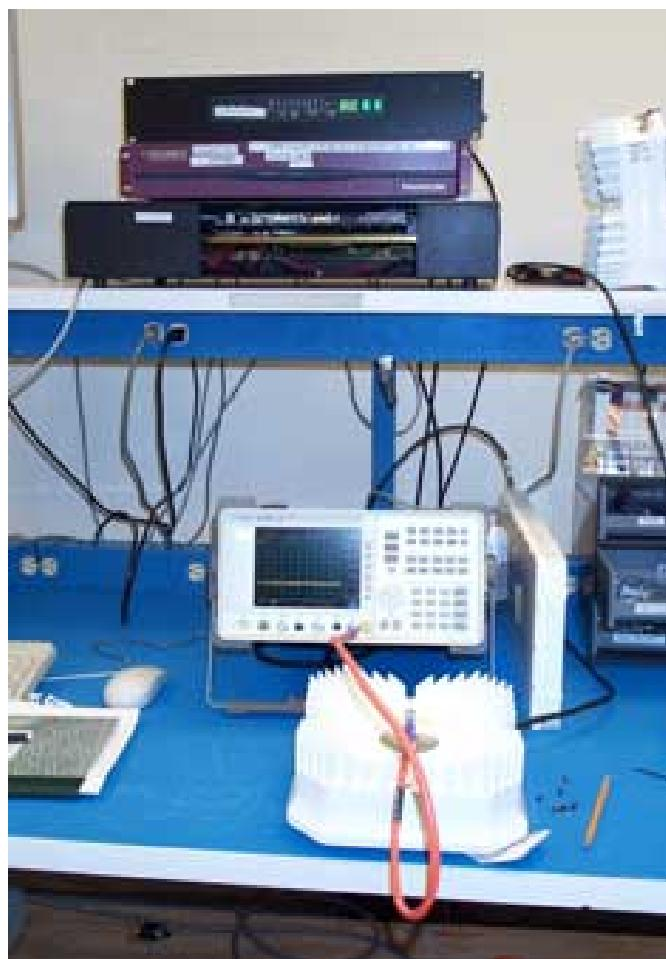
Figure 5 CPE ODU 9 kHz-200 GHz Test Set Up
