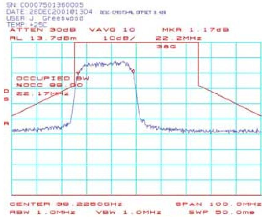
CPE088: Occupied Bandwidth (CPE-ODU) 39.2375 GHz 16QAM:
