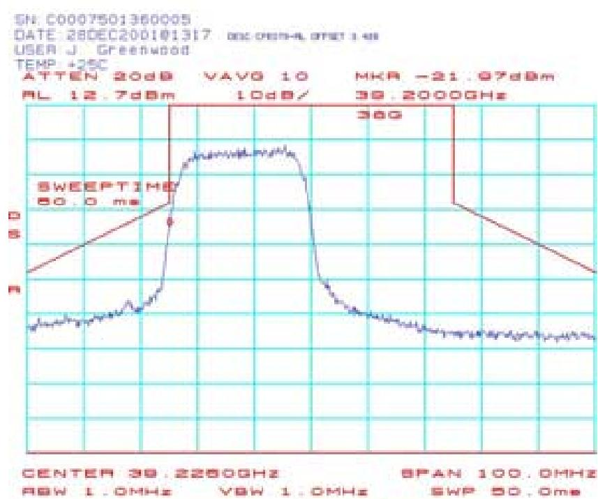
**CPE080: Spectrum Mask Plots (CPE-ODU) 39.2125 GHz 64QAM:**
