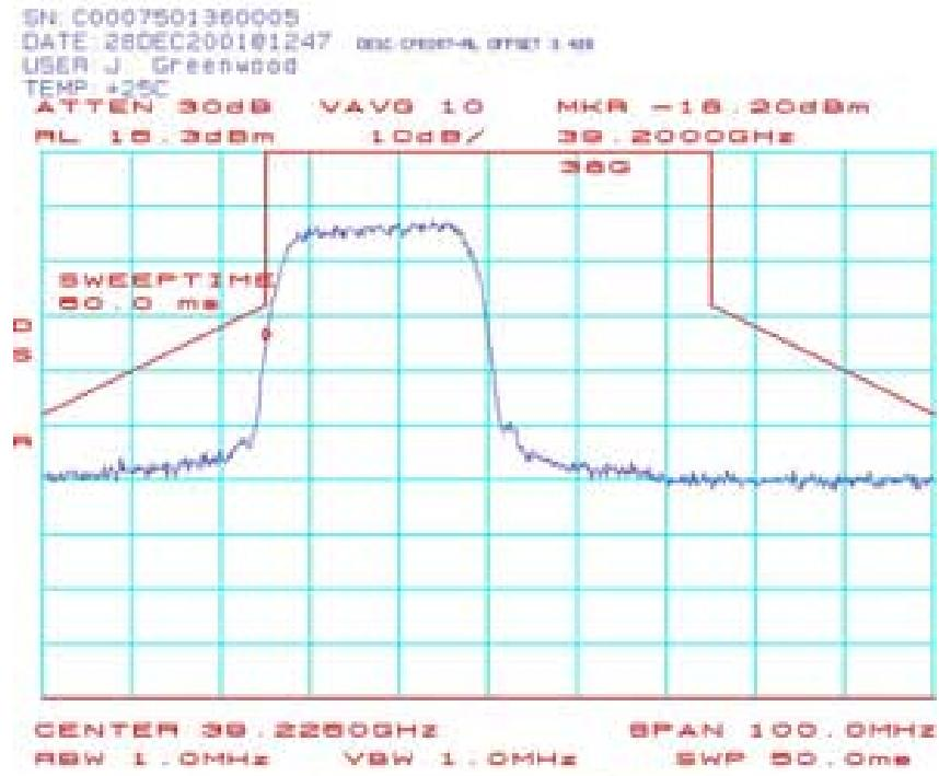
CPE072: Spectrum Mask Plots (CPE-ODU) 39.2125 GHz 16QAM:
