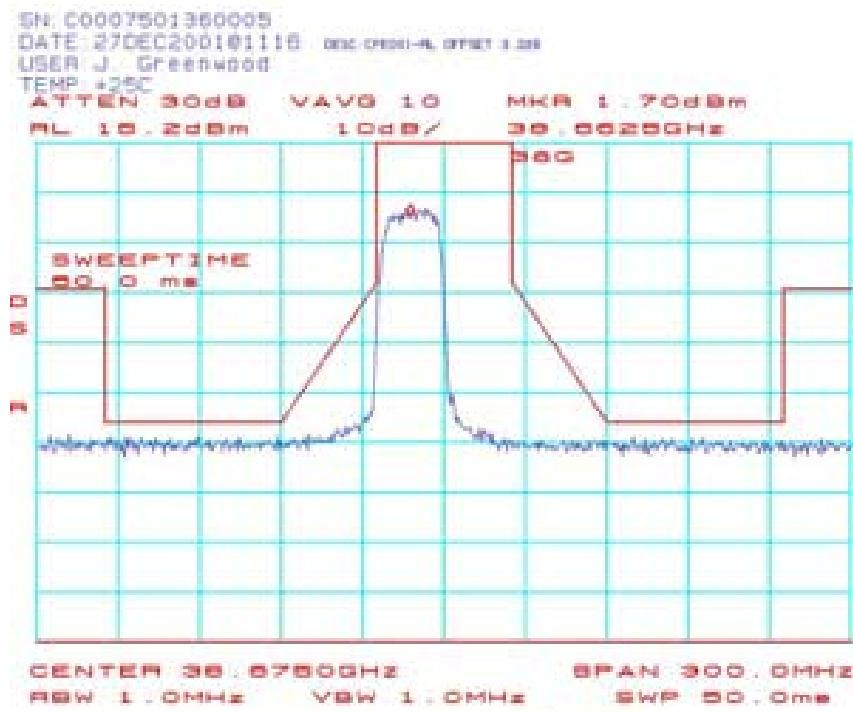
**CPE002: Spectrum Mask Plots (CPE-ODU) 38.6625 GHz QPSK:**
