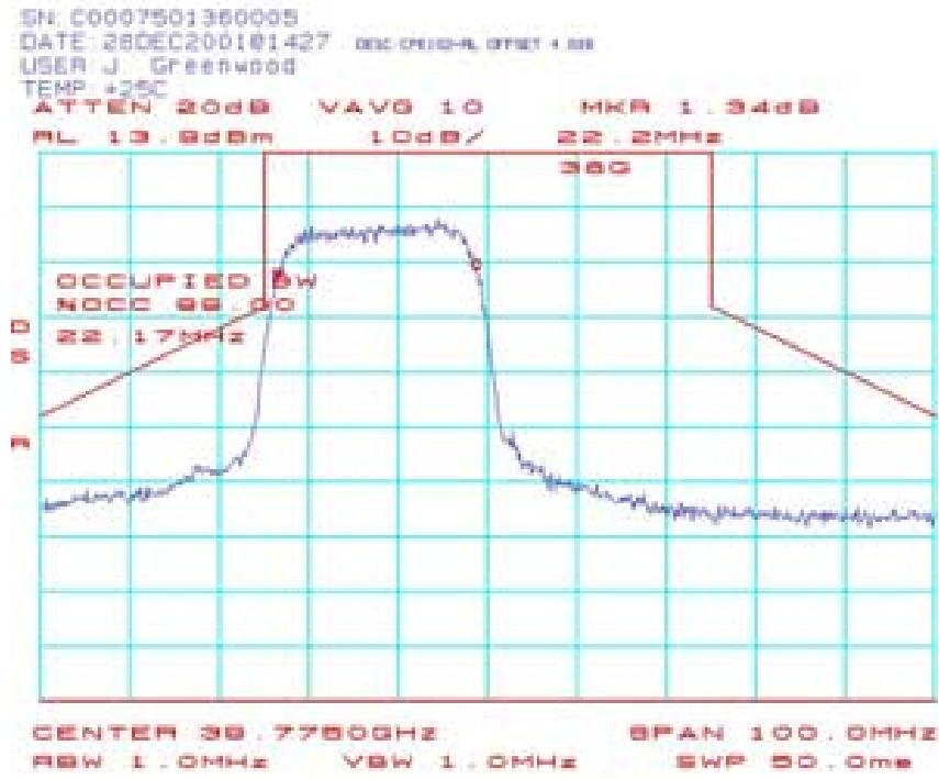
CPE119: Occupied Bandwidth (CPE-ODU) 39.7875 GHz 16QAM:
