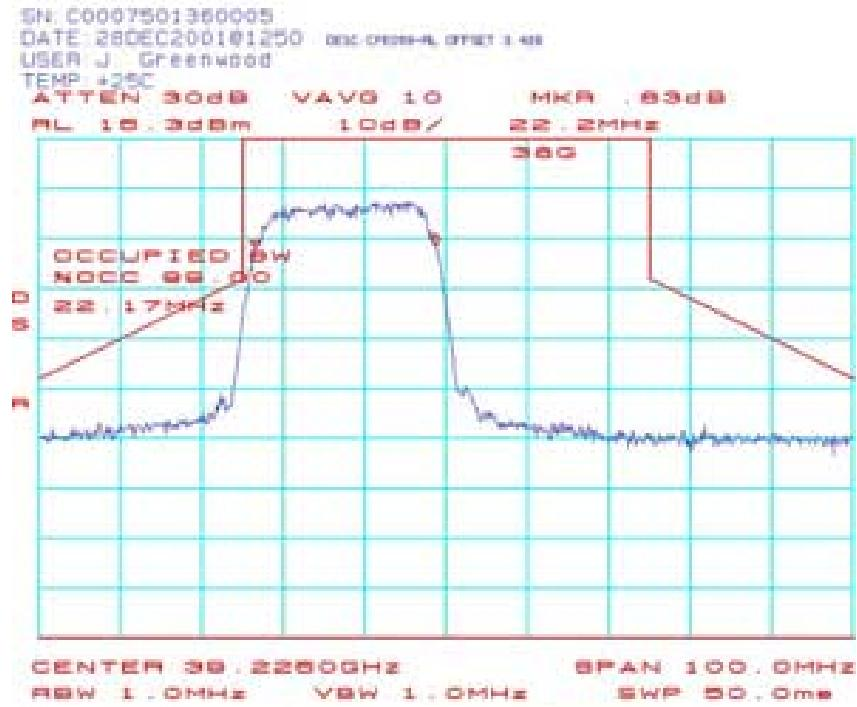
**CPE084: Occupied Bandwidth (CPE-ODU) 39.2375 GHz QPSK:**
