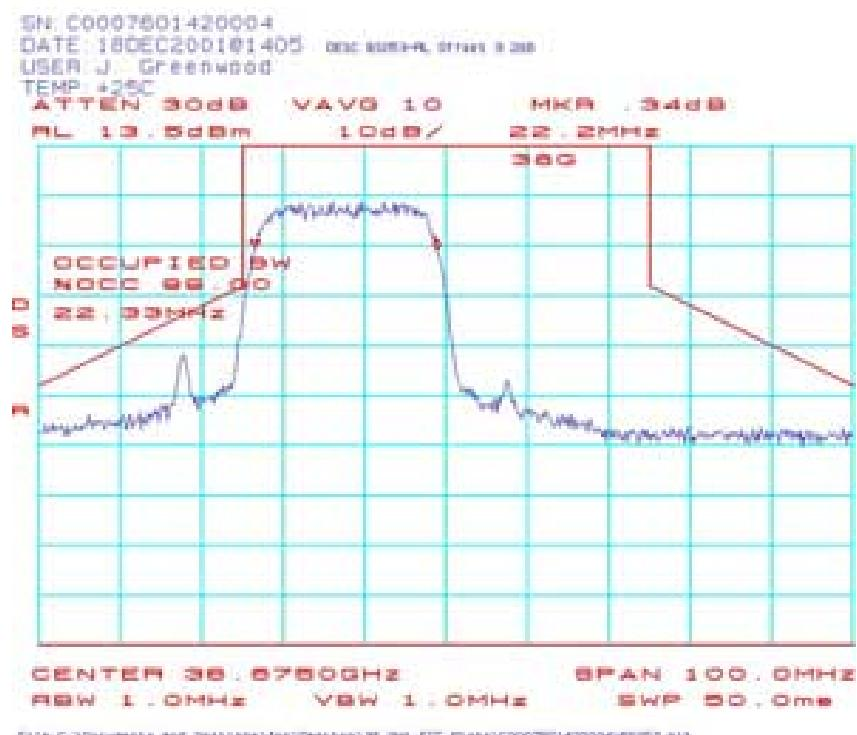
**BS067: Occupied Bandwidth (BS-ODU) 38.6875 GHz 16QAM:**
