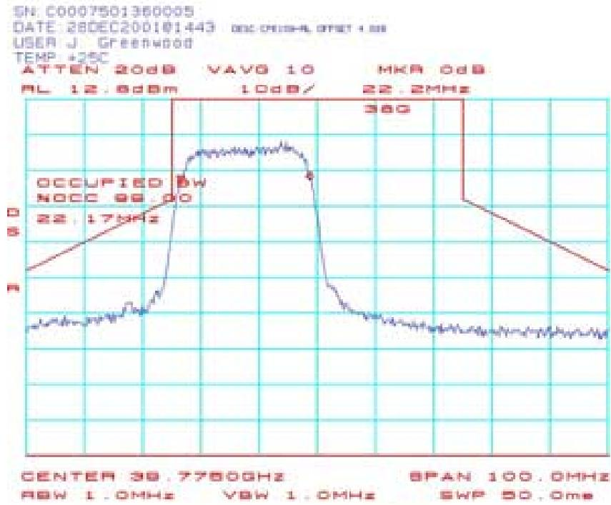
**CPE125: Occupied Bandwidth (CPE-ODU) 39.7875 GHz 64QAM:**
