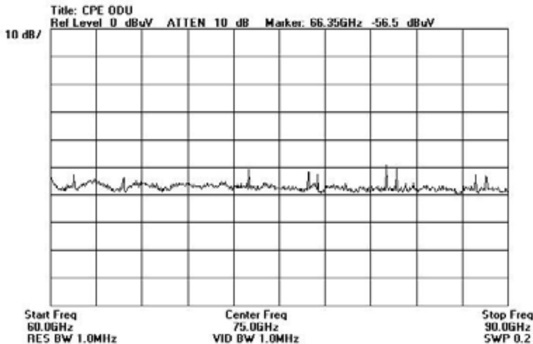
Note: the plots read dBuV but the actual measurement is in dBm. This is due to a limitation in the software used to capture the plots.
