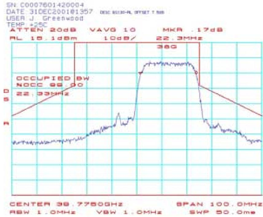
**BS118: Occupied Bandwidth (BS-ODU) 39.7625 GHz 16QAM:**
