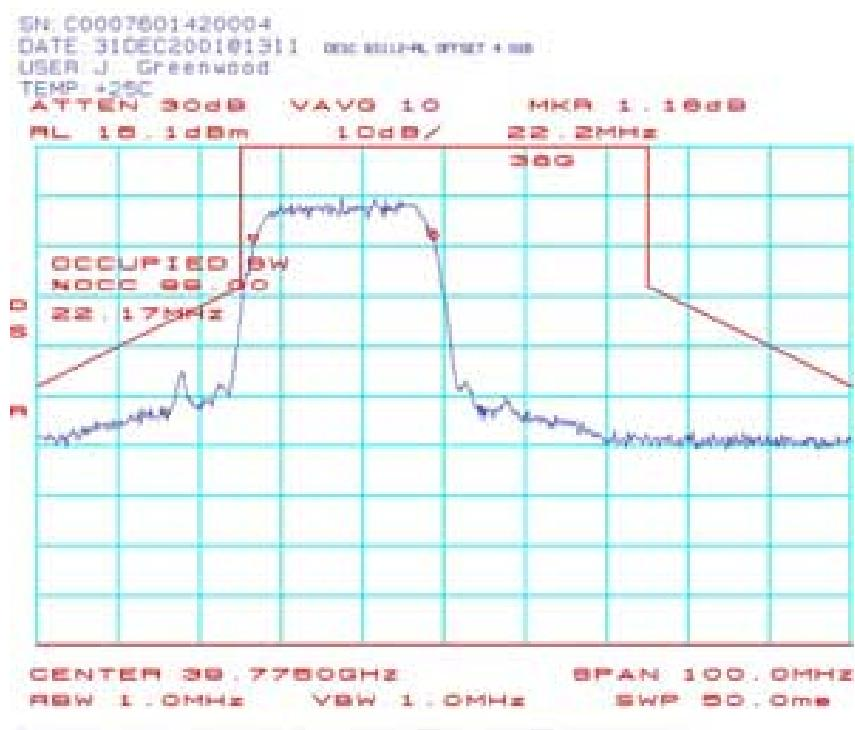
**BS130: Occupied Bandwidth (BS-ODU) 39.7875 GHz QPSK:**
