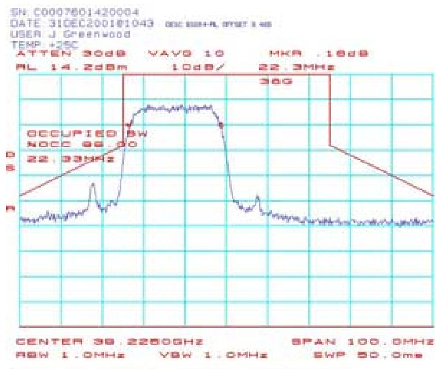
**BS102: Occupied Bandwidth (BS-ODU) 38.2375 GHz 16QAM:**
