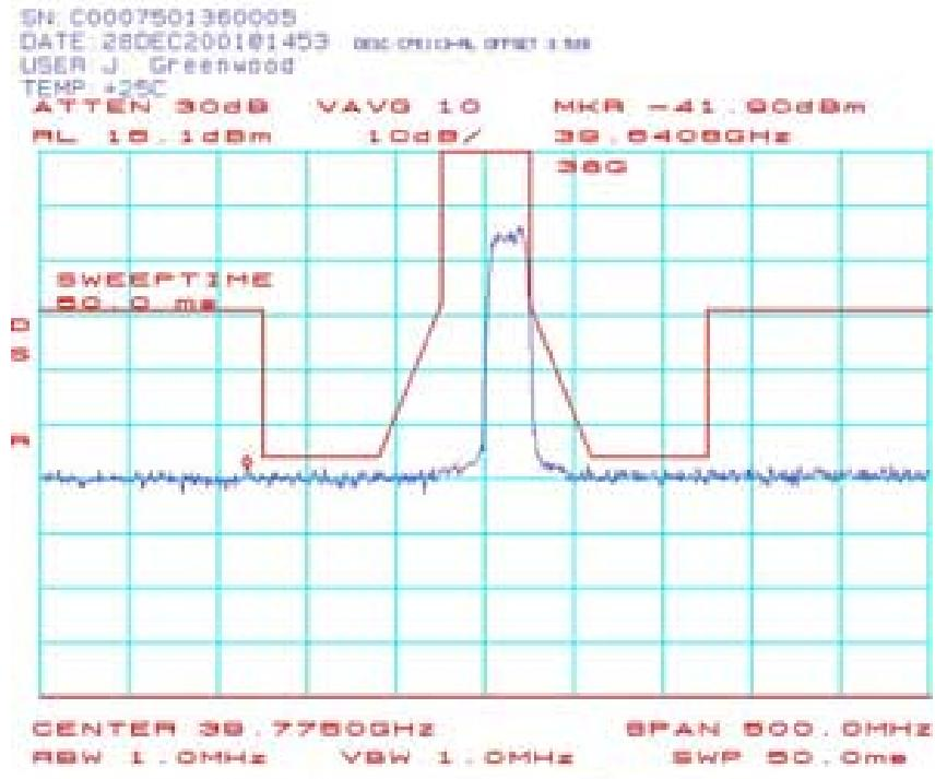
CPE114: Spectrum Mask Plots (CPE-ODU) 39.7875 GHz QPSK:
