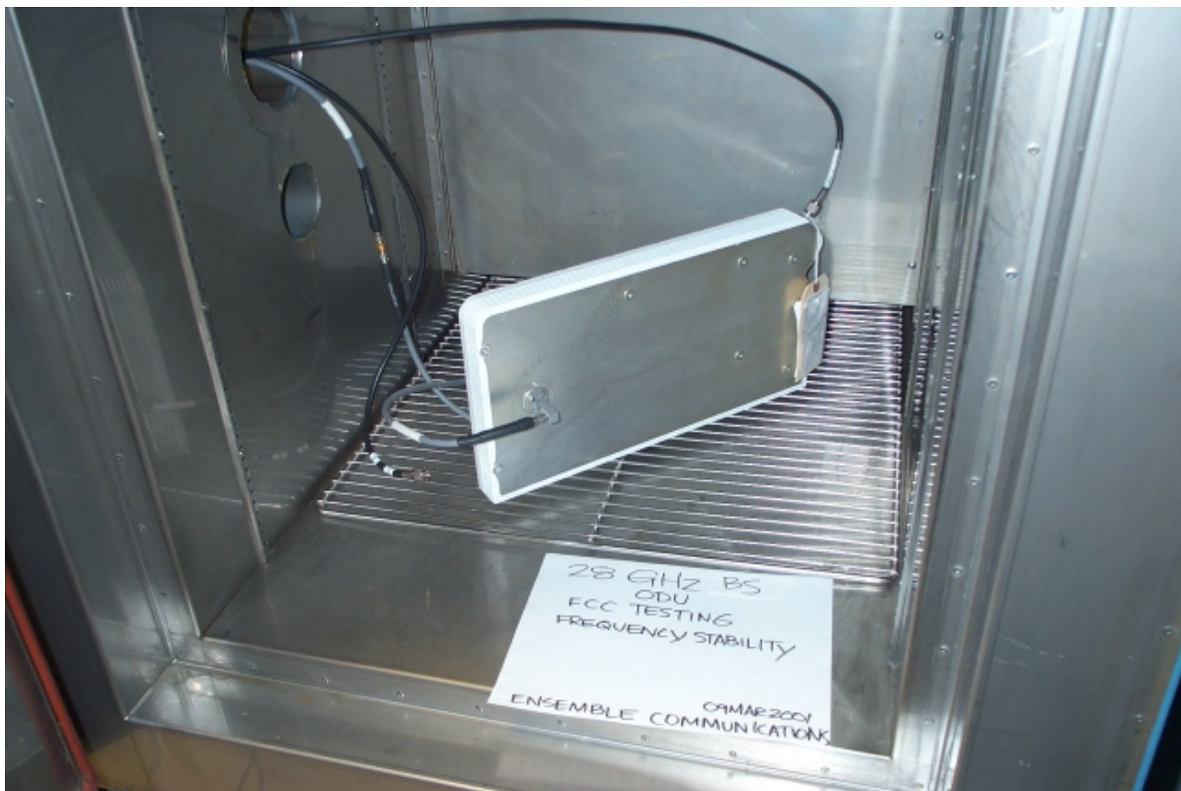
BS-ODU Test Hook-up in Temperature Chamber
