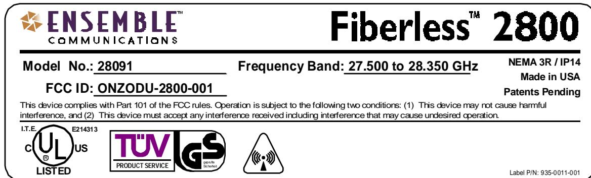
BS-ODU Regulatory Label - 1.5" x 5", 90 degree sector antenna, vertically polarized
