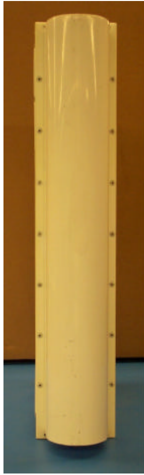
Base Station ODU, with antenna Front view
