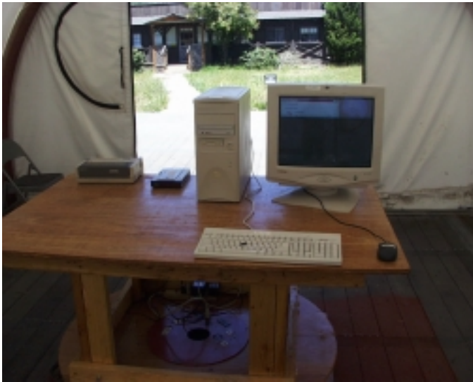
Radiated Emission Setup Photos (Worst Emission Position)
