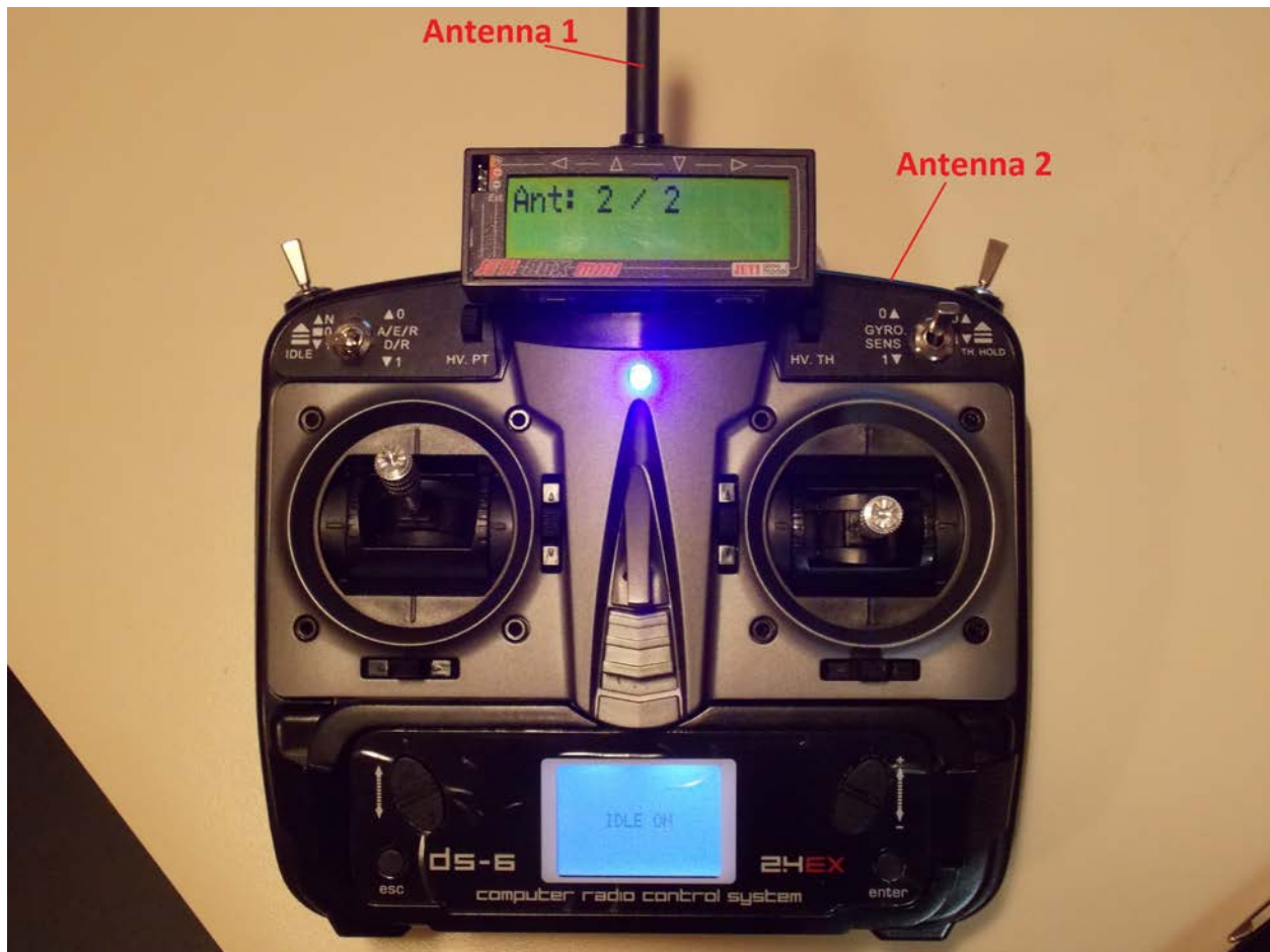
Front of Device and Antenna Location
