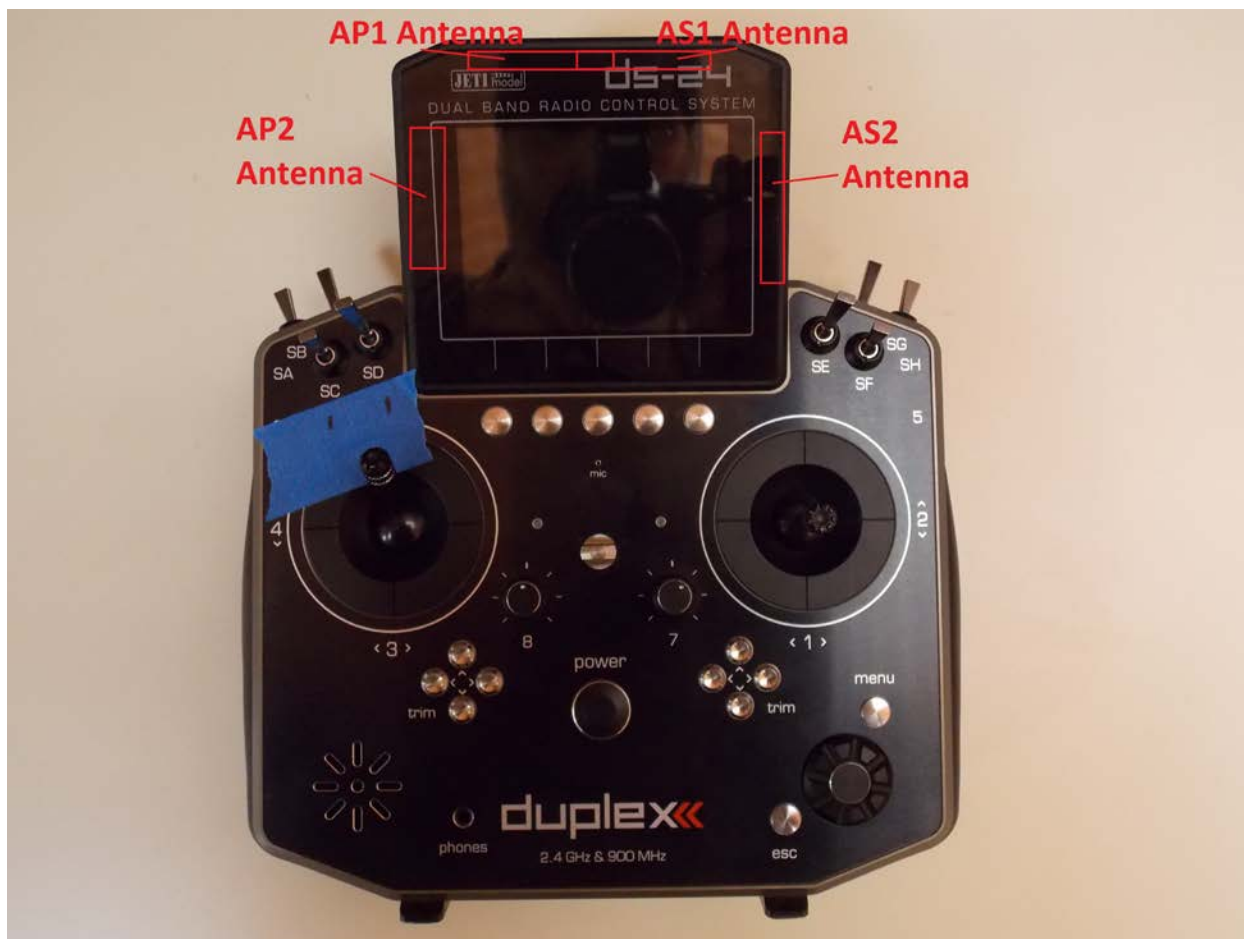
Front of Device and 2.4 GHz Antenna Location
