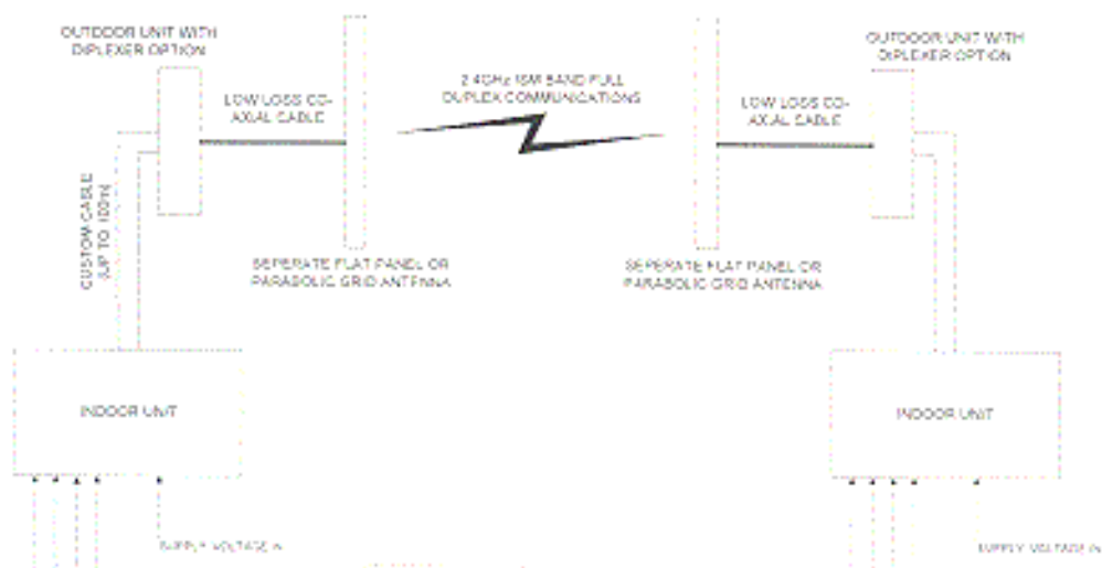
Figure 2: Outdoor Unit with Internal Diplexer and Seperate Antenna
