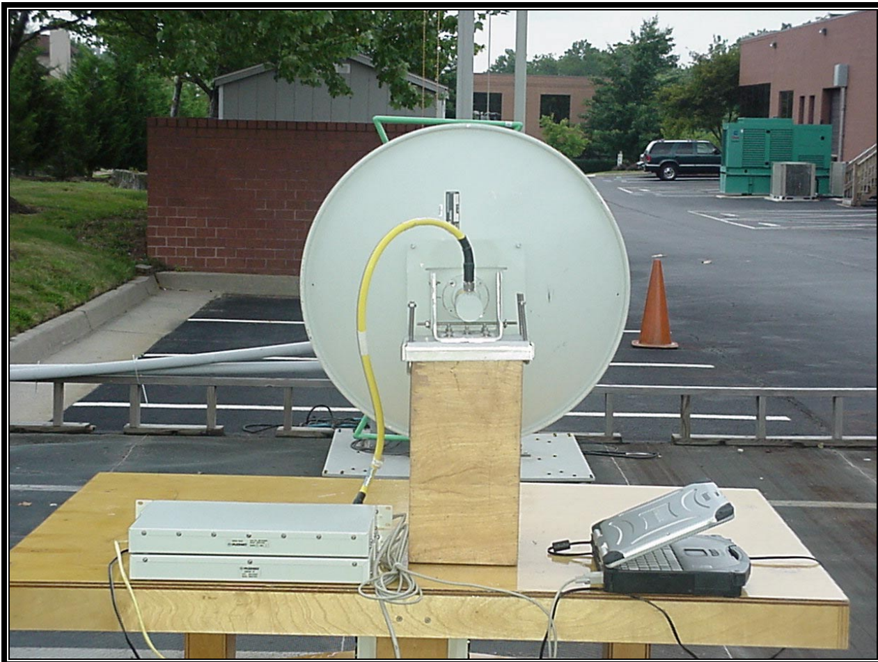
PHOTOGRAPH 2: RADIATED EMISSIONS REAR VIEW - PARABOLIC ANTENNA
