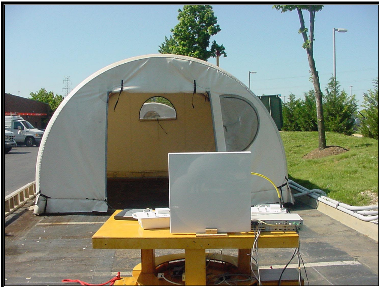
PHOTOGRAPH 3: RADIATED EMISSIONS FRONT VIEW – FLAT PANEL ANTENNA
