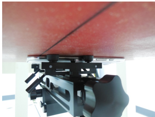
Band850, Band1900, WCDMA Band II/V Test Setup Body Back with gap 0mm
