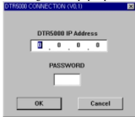
Enter the DTR5000N IP address and password (or if you changed the IP address, enter the new one) and click OK. Then “dtr\_conn” will automatically transfer the Filter IP and Destination IP to DTR5000N.
