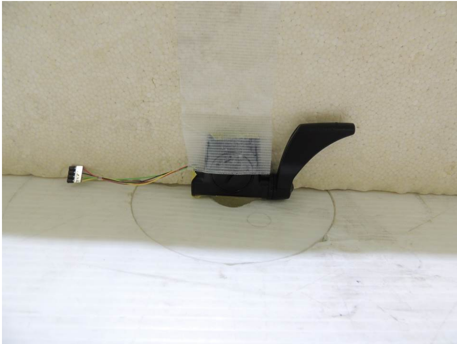
Photograph 5: Set-up for Radiated Emission, EUT Configuration Y-Axis
