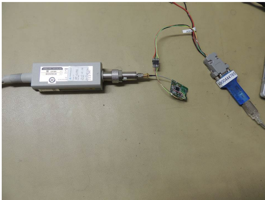
Photograph 1: Set-up for Conducted Emissions at Antenna Port
