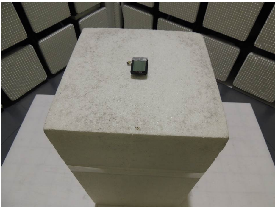
Photograph 2: Set-up for Radiated Emission of Transmitter, Front View
