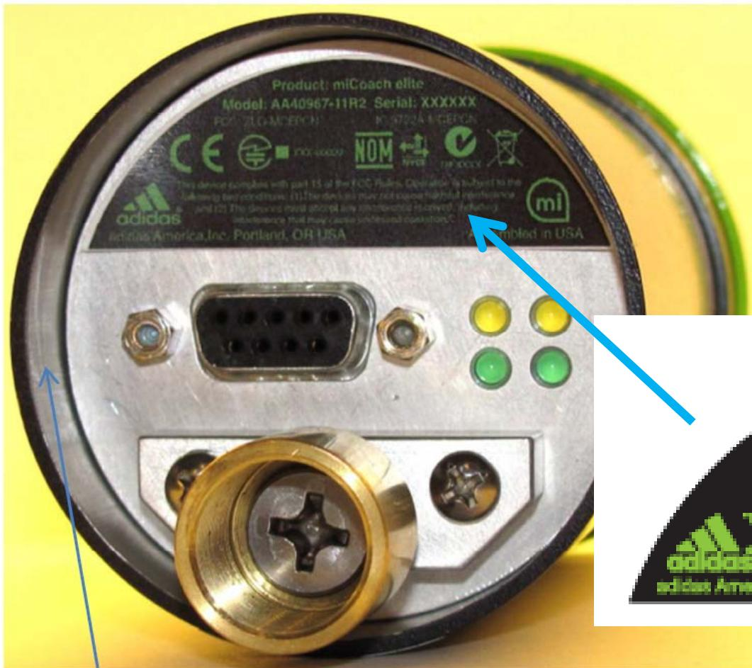
Bar Code Label can be placed here on inside lip for tracking purposes.
