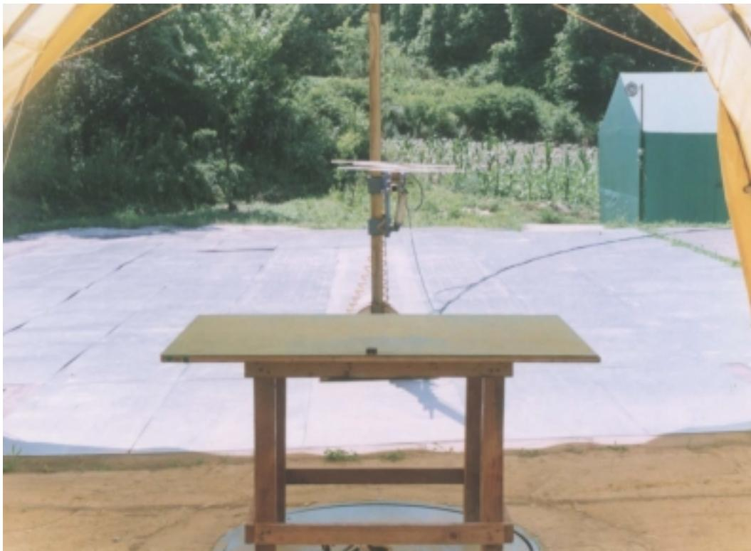
**FIGURE D-1. WORST-CASE RADIATED EMISSIONS TEST SETUP**
