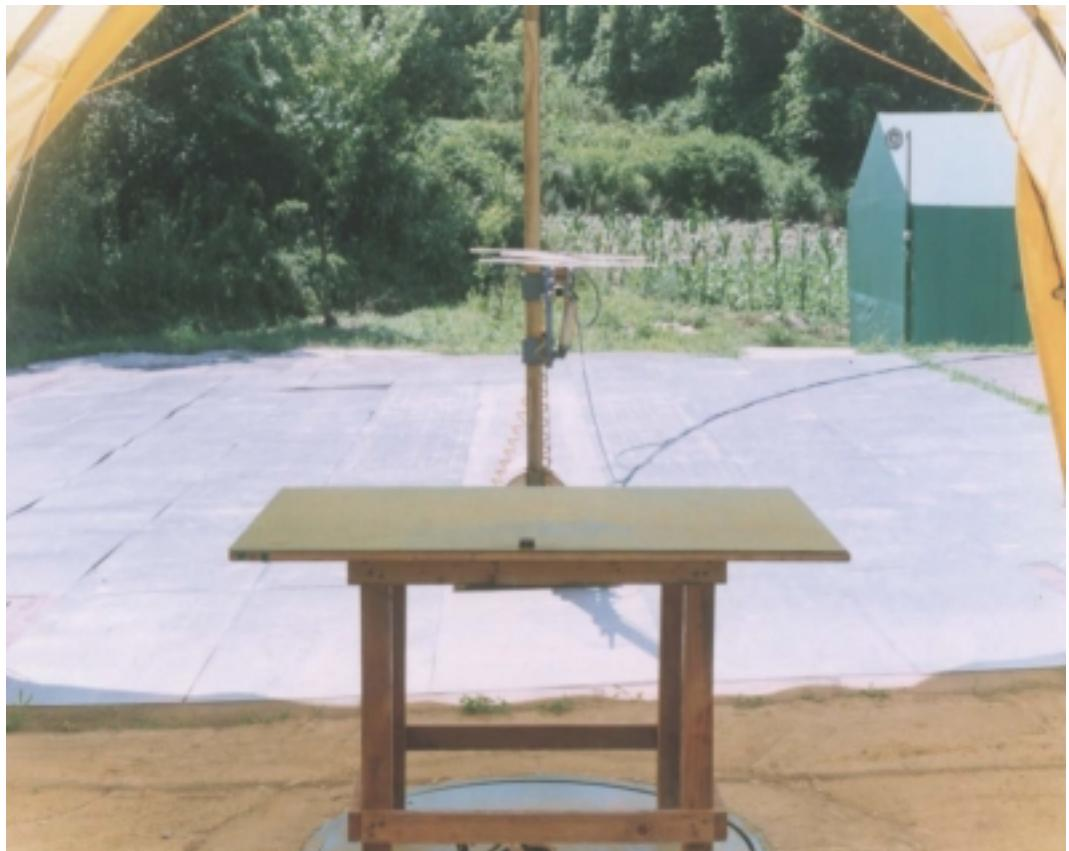
**FIGURE D-1. WORST-CASE RADIATED EMISSIONS TEST SETUP**
