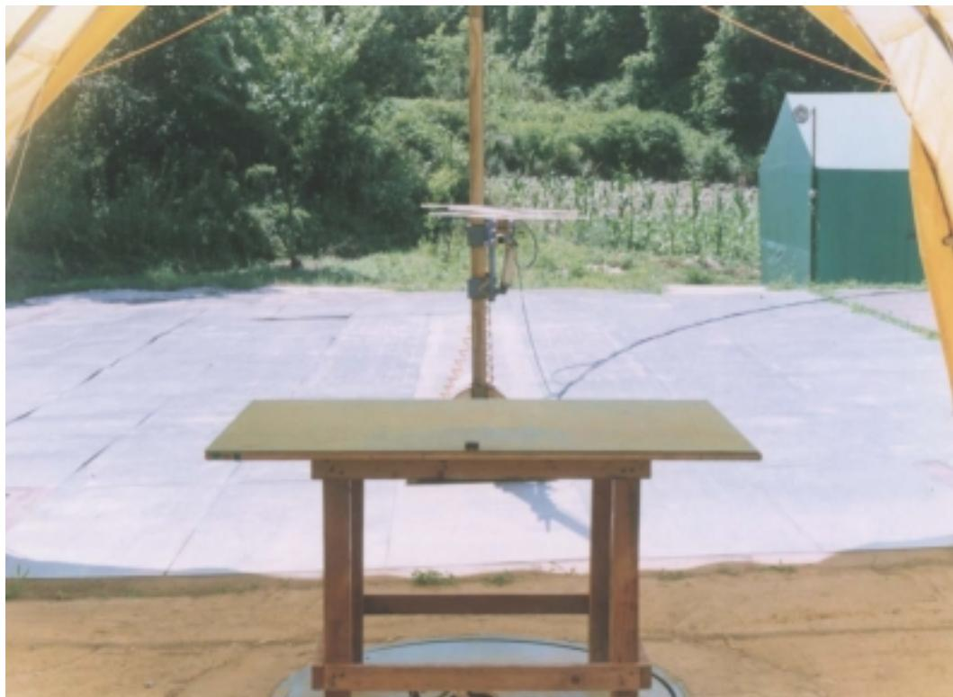
**FIGURE D-1. WORST-CASE RADIATED EMISSIONS TEST SETUP**
