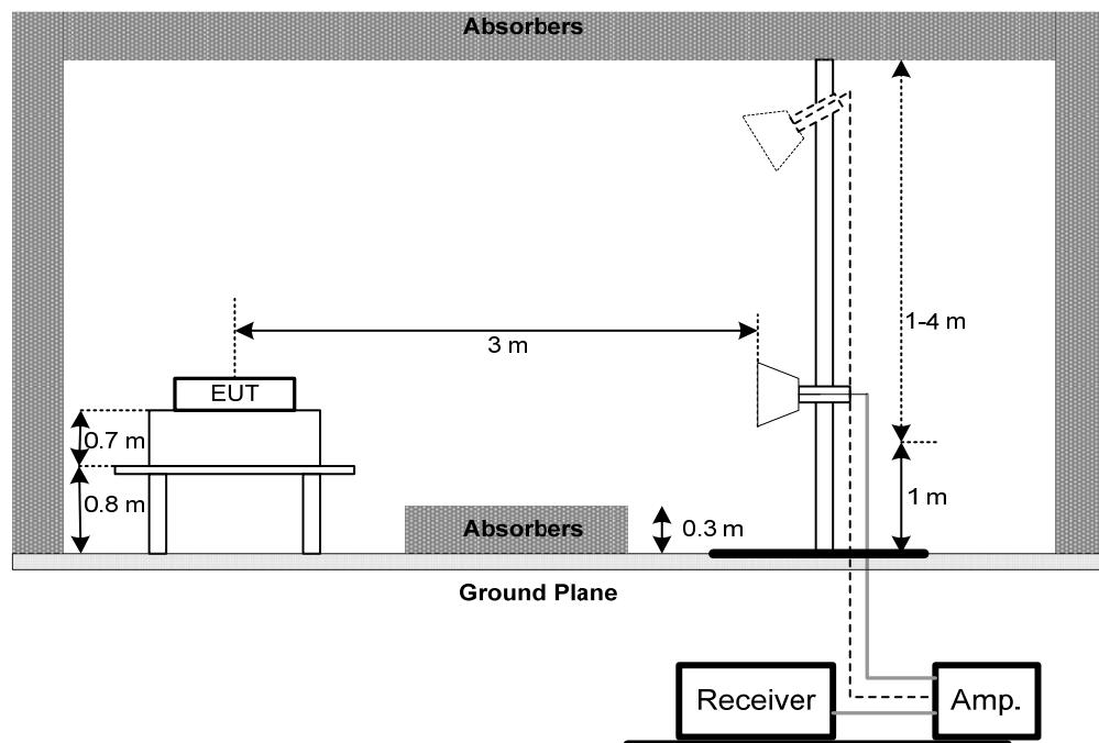
(C) For radiated emissions below 30MHz
