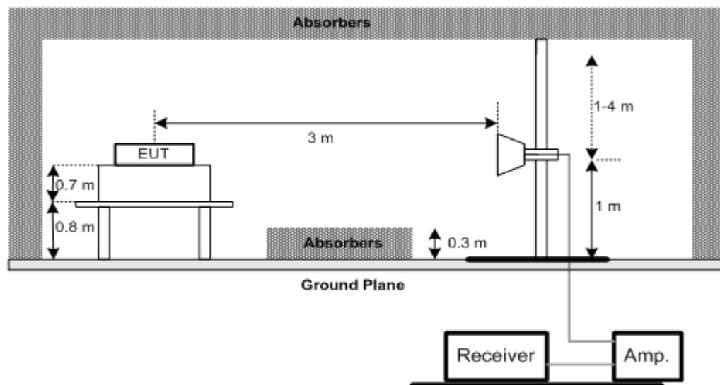
(C) For radiated emissions below 30MHz
