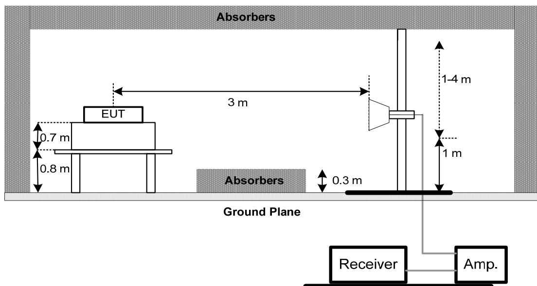
(C) For radiated emissions below 30MHz
