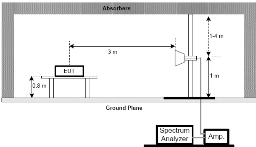
(C) For radiated emissions below 30MHz
