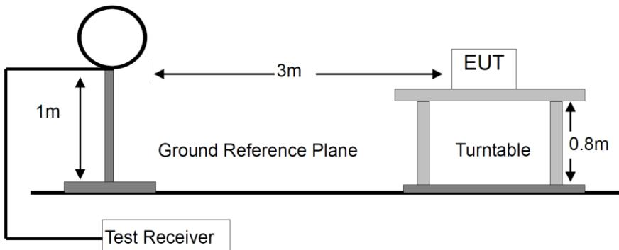
For Radiated Emission 30-1000MHz
