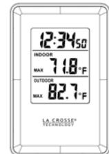
**RESET:** Hold the MAX/MIN key for 2 seconds to manually clear all the MIN/MAX records.
