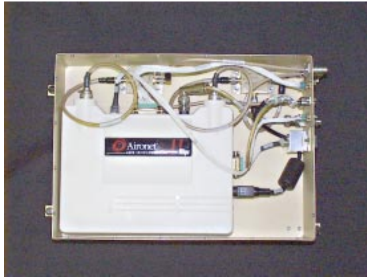
Figure 5: Access Point Showing Internal Chassis Design
