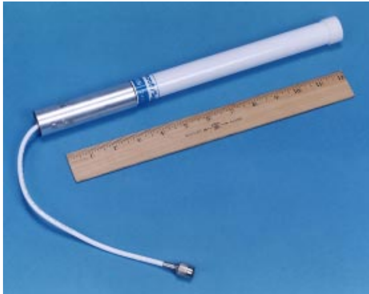
Figure 5: Ground Segment (Access Point) Antenna
