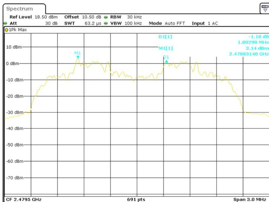
**EDR (8DPSK): Low Channel**
