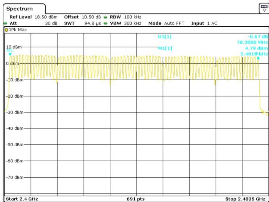
**EDR ( $\pi/4$ -DQPSK): Number of Hopping Channels**
