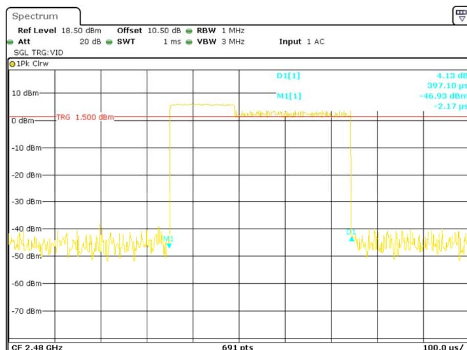
**Pulse time, Low Channel, 2DH3**
