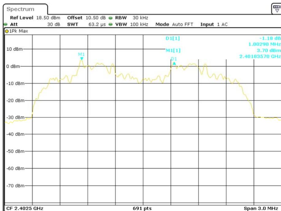
**EDR ( $\pi/4$ -DQPSK): Middle Channel**
