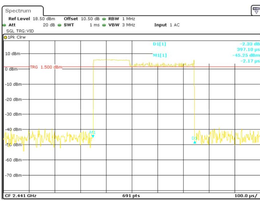
**Pulse time, High Channel, 3DH1**
