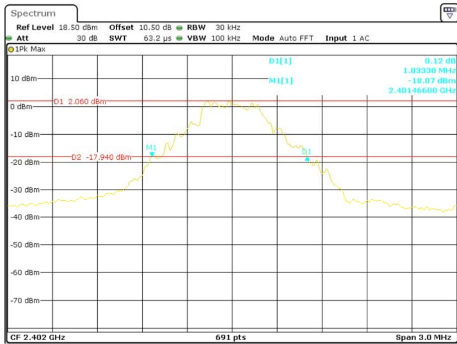
**BDR (GFSK): Middle Channel**
