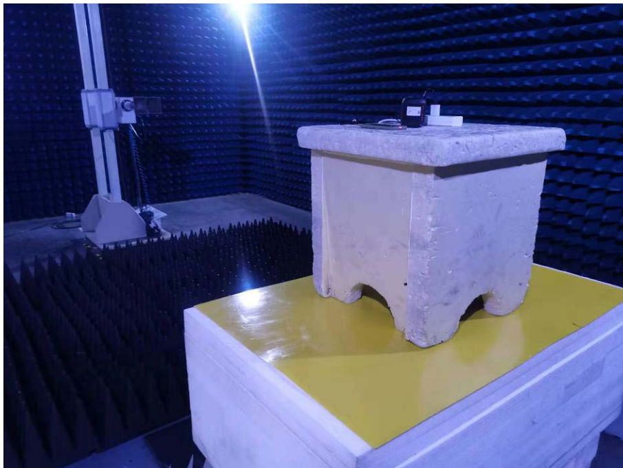
Photo of Radiated Emission Measurement Above 1GHz
