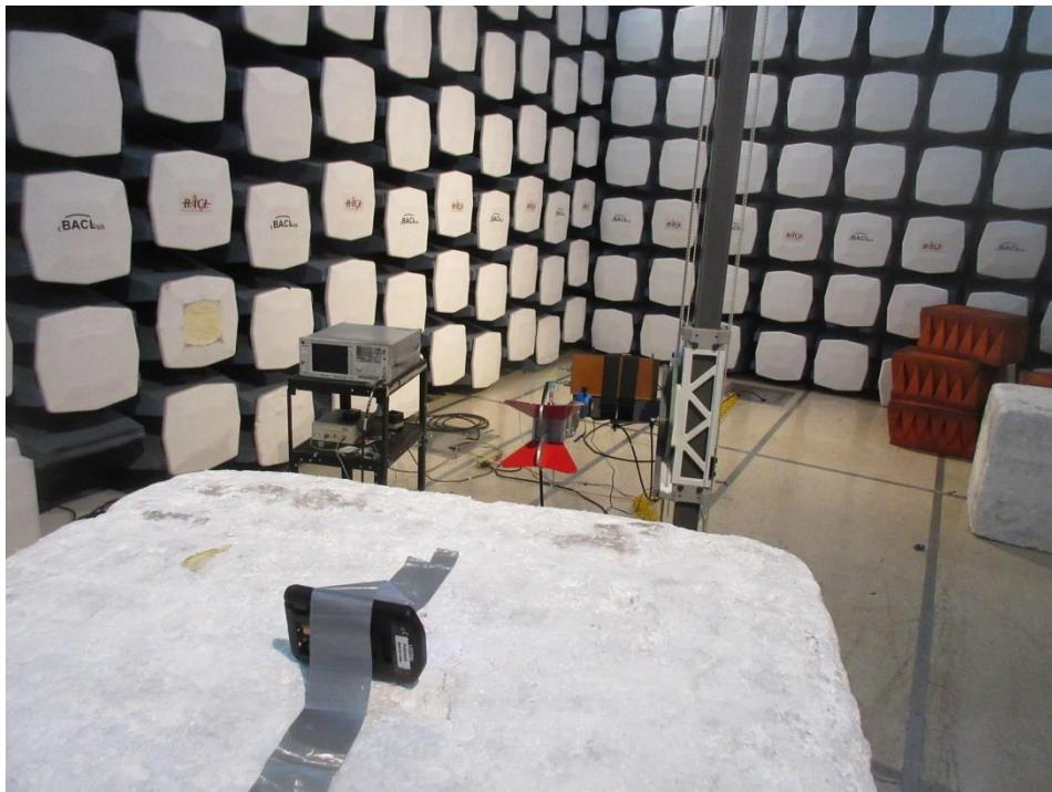
**1.7 18 – 26.5 GHz at 1 Meter Front View**
