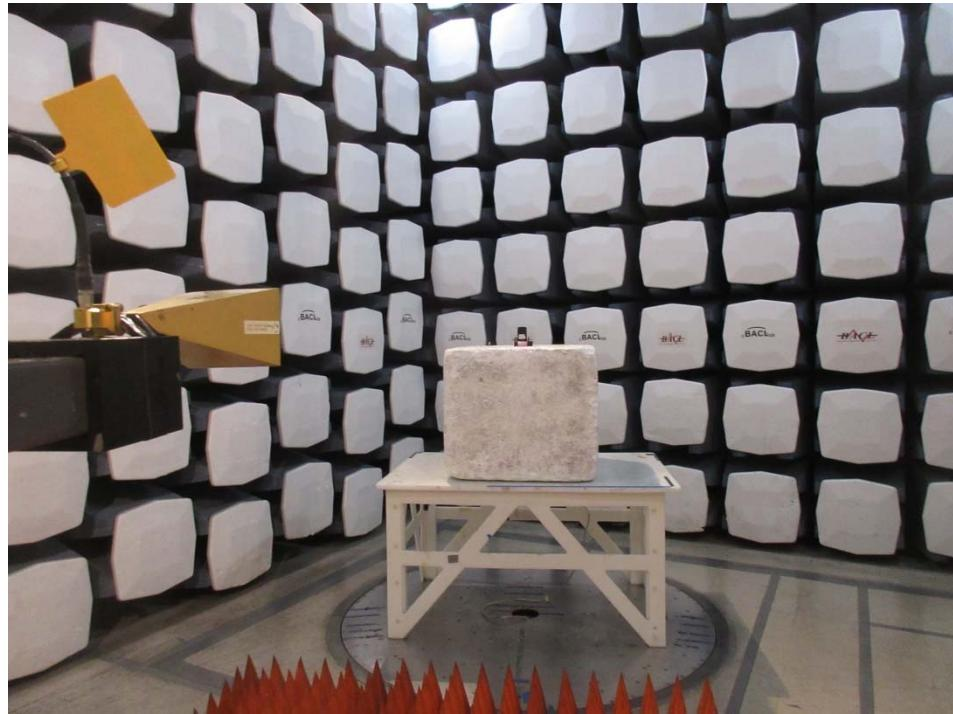
**1.6 Radiated Spurious Emissions: 18 GHz to 26.5 GHz, Rear View at 3 meters distance**
