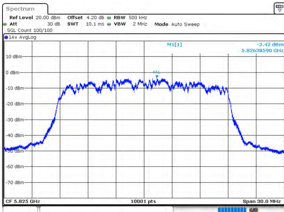
PSD NVNT ac20 5825MHz Ant2
