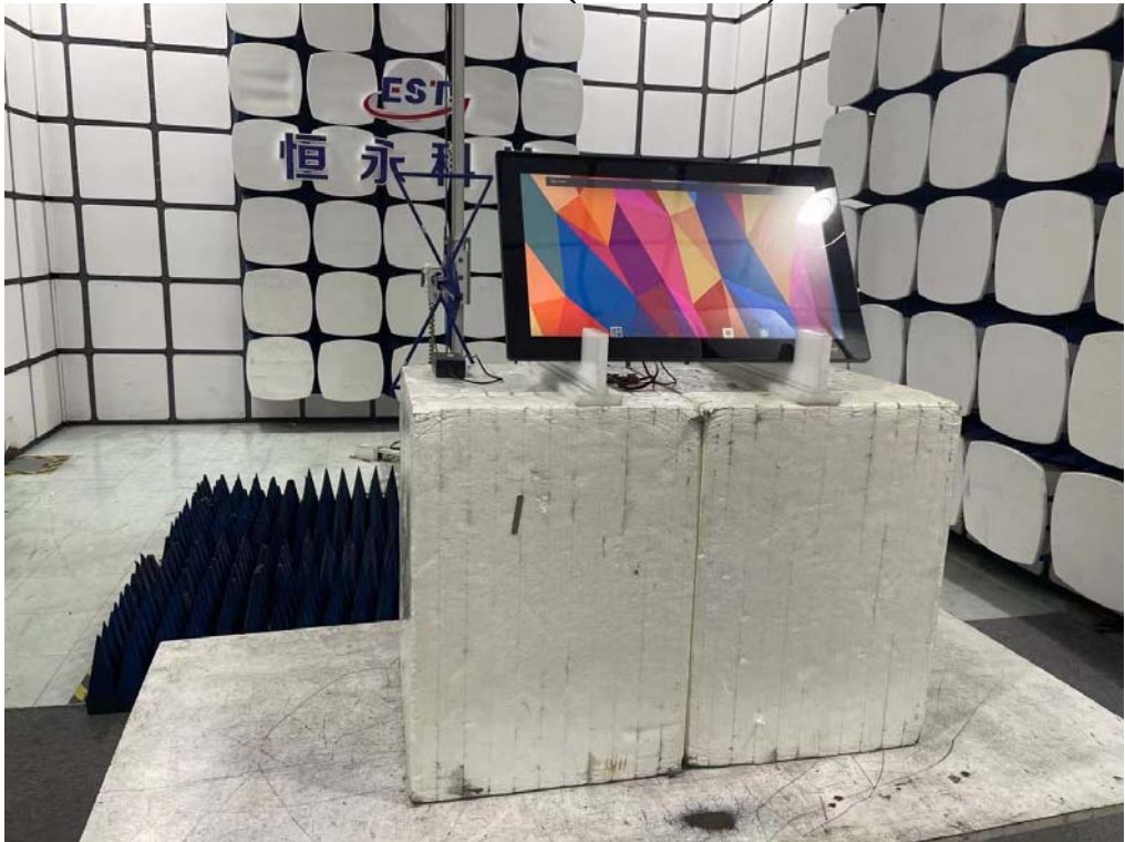
Radiated Test (Below 1GHz)
