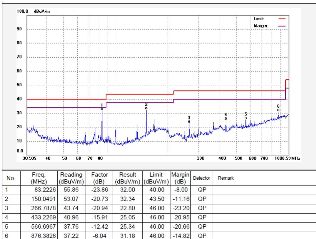
Remark: Factor = Antenna factor + cable loss – preamplifier gain
