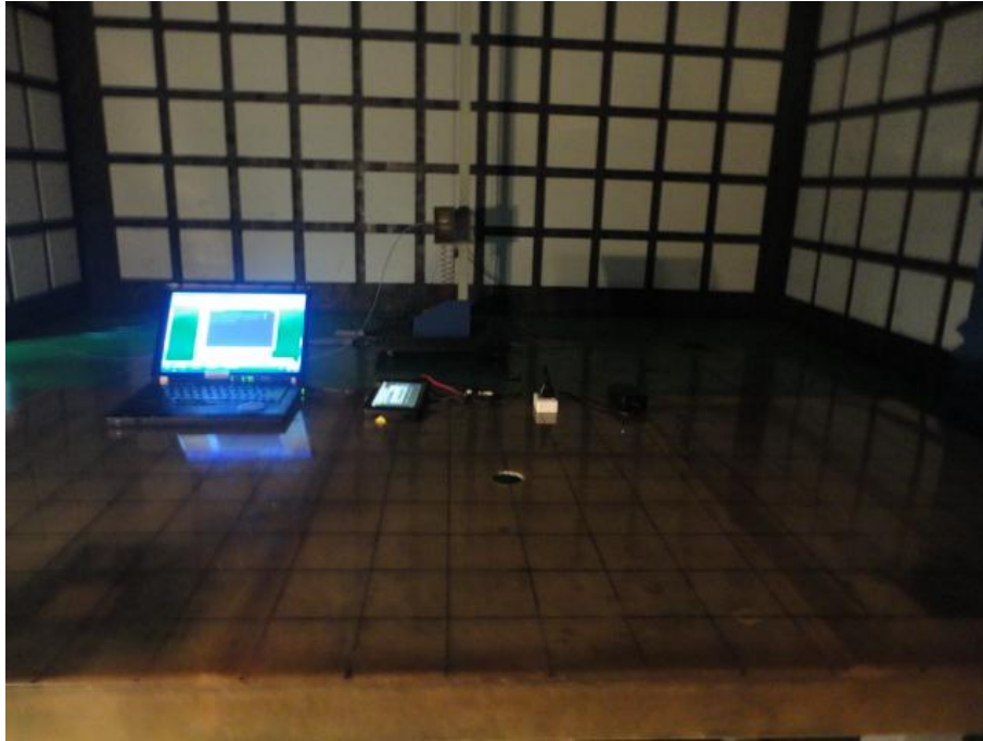
Radiated Emission Test Above 1GHz
