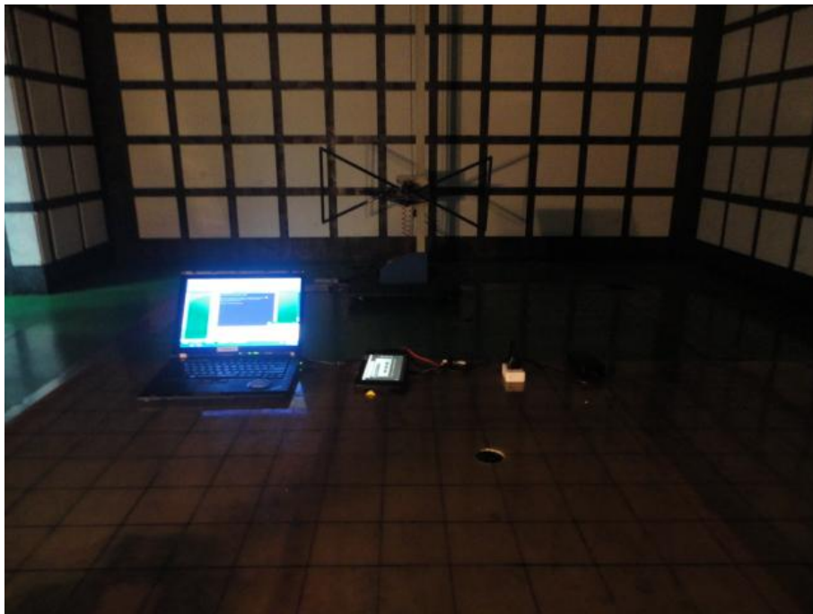
Radiated Emission Test Below 1GHz
