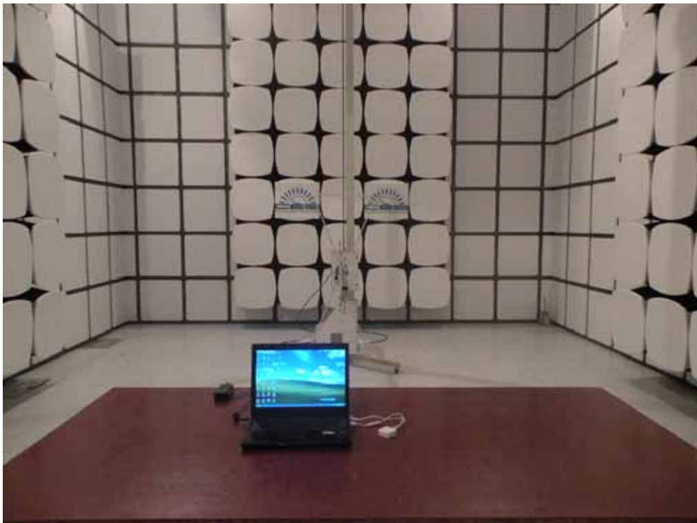
Radiated Emission Test Setup in Chamber
