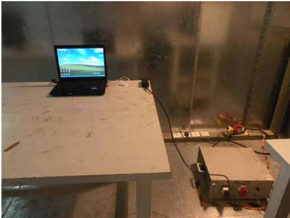
Radiated Emission Test Setup in Chamber
