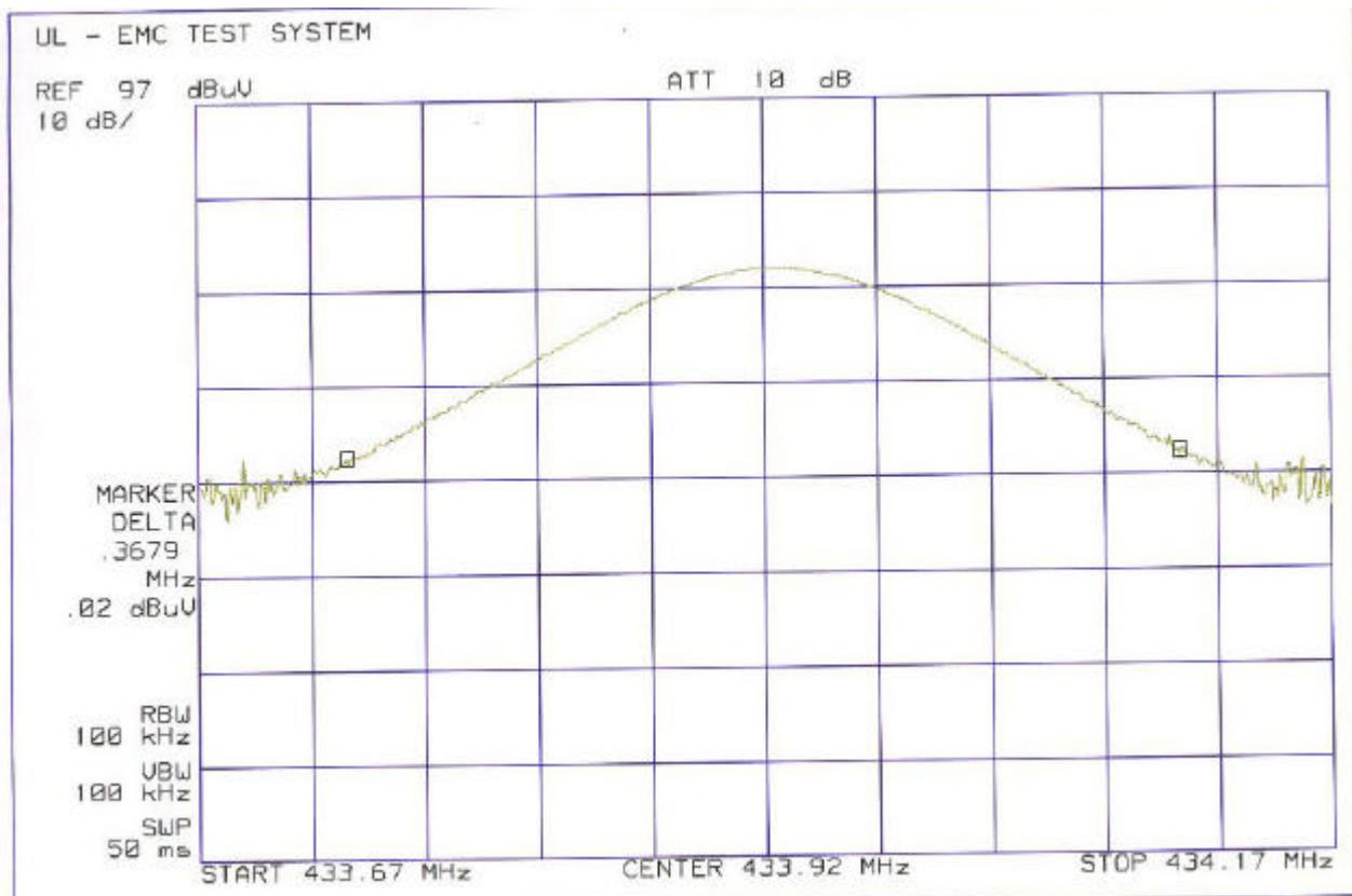
Per RSS-210 clause 6.1.1(c) and CFR 47, Part 15 clause 15.231(c), the 20dB bandwidth shall be no wider than 0.25% of the center frequency for devices operating above 70MHz and below 900MHz.
