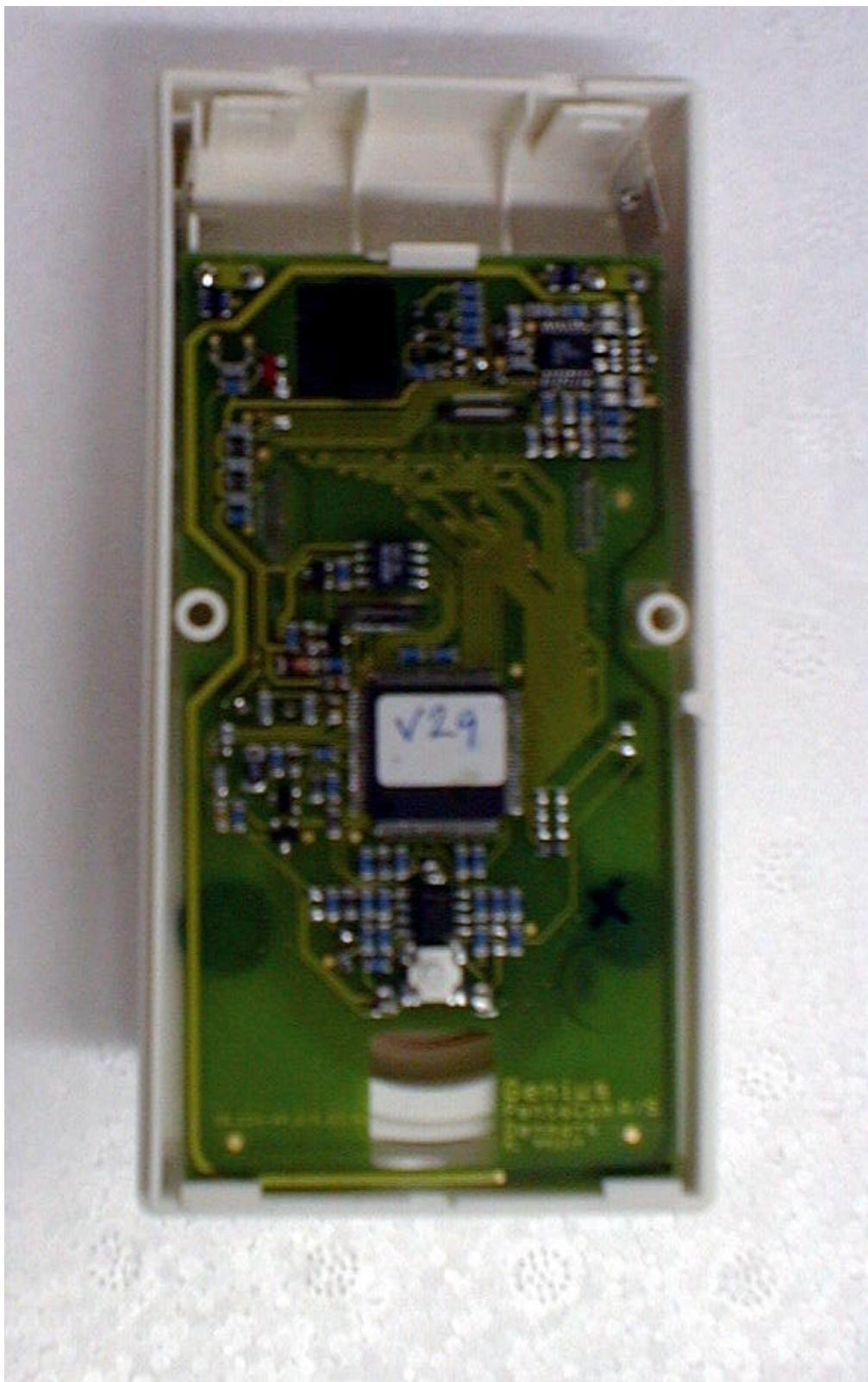
**EUT Internal – Front of PWB**
