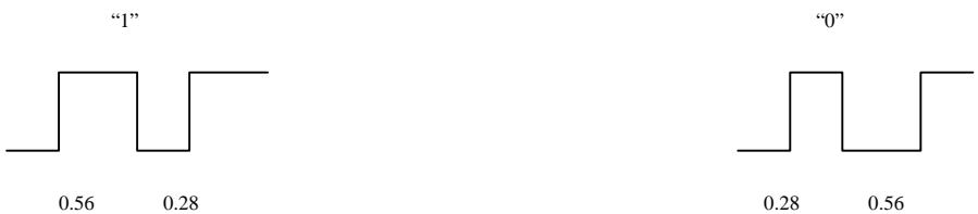
c. The frame: Occupy 17 bits, being made up of 1 bit start code and 16 bits data code.
