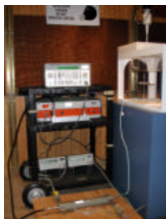
Figure A.0 Dipole Validation Test Setup
