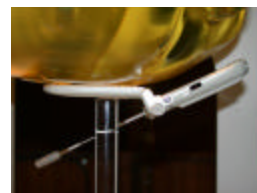
Figure A.1 Right Head SAR Test Setup -- Cheek / Touch Position --
