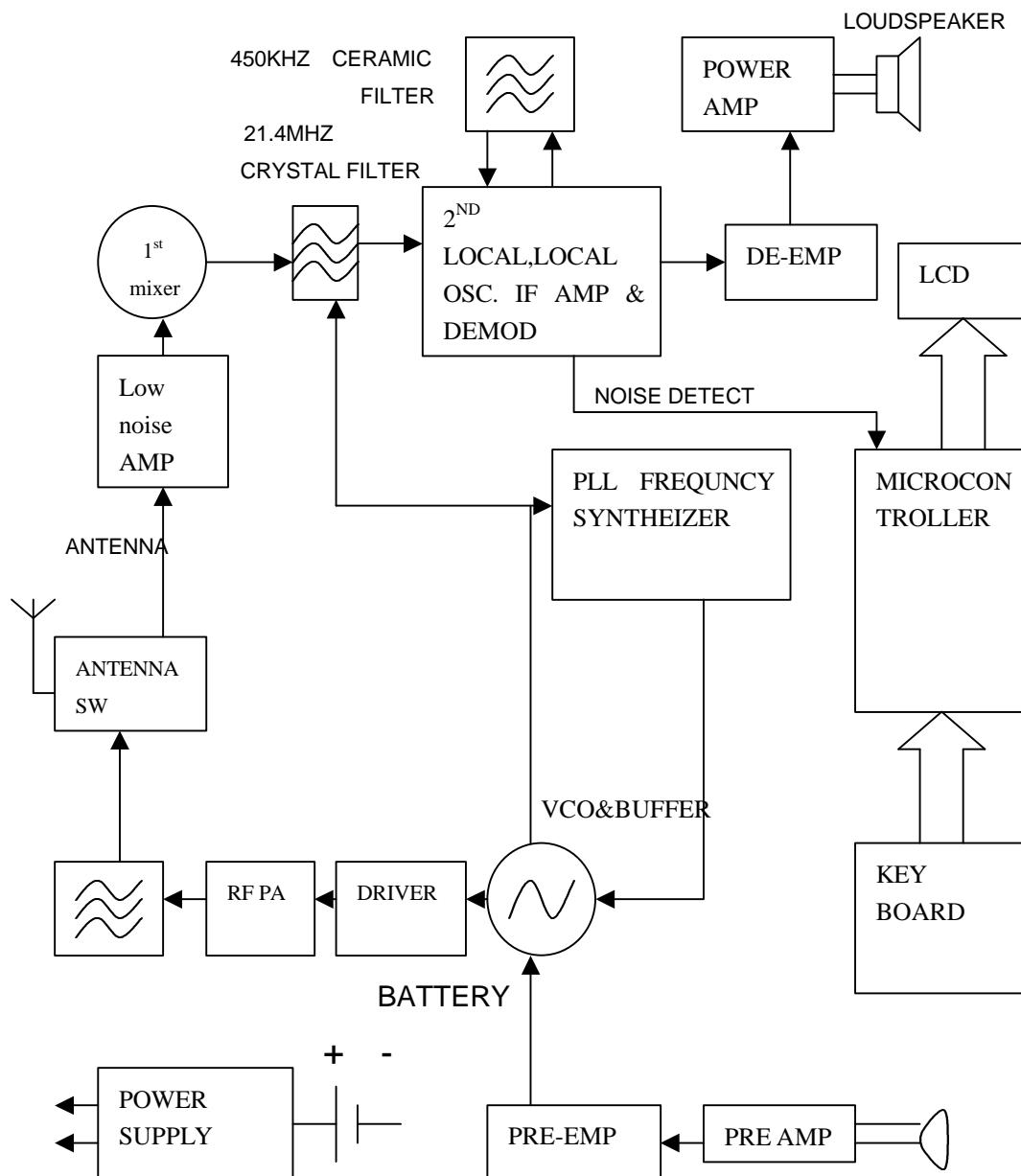
As is evident in the above block diagram, this product employs dual-conversion superhet architecture for its receiver. The first IF (Intermediate Frequency) is 21.4MHz. The second IF is 450kHz. The local oscillator signal is PLL-synthesized to ensure accuracy and stability. A microcontroller with appropriate firmware is designed to program the PLL to the desirable user-selected channel for either transmit or receive.
