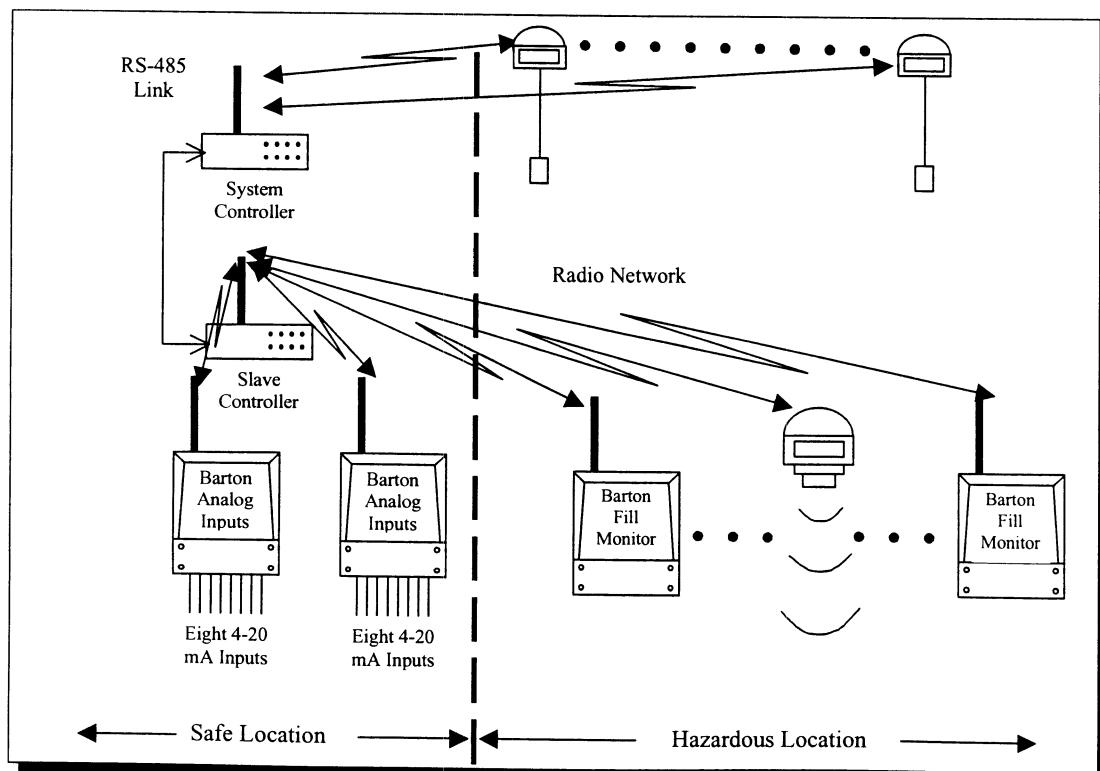
This illustration depicts a W-Series TankScan local RF network. The **WC** controller can communicate with up to 30 **WL** monitors, **WF** indicators or **WA** Analog Input Monitors up to 500 feet away. Data is relayed to the Host system via dial-up telephone or other means.
