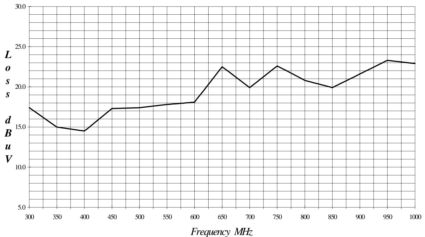
**PREAMPLIFIER EFFECTIVE GAIN AT 3 METERS PA-102 S/N: 1414**
