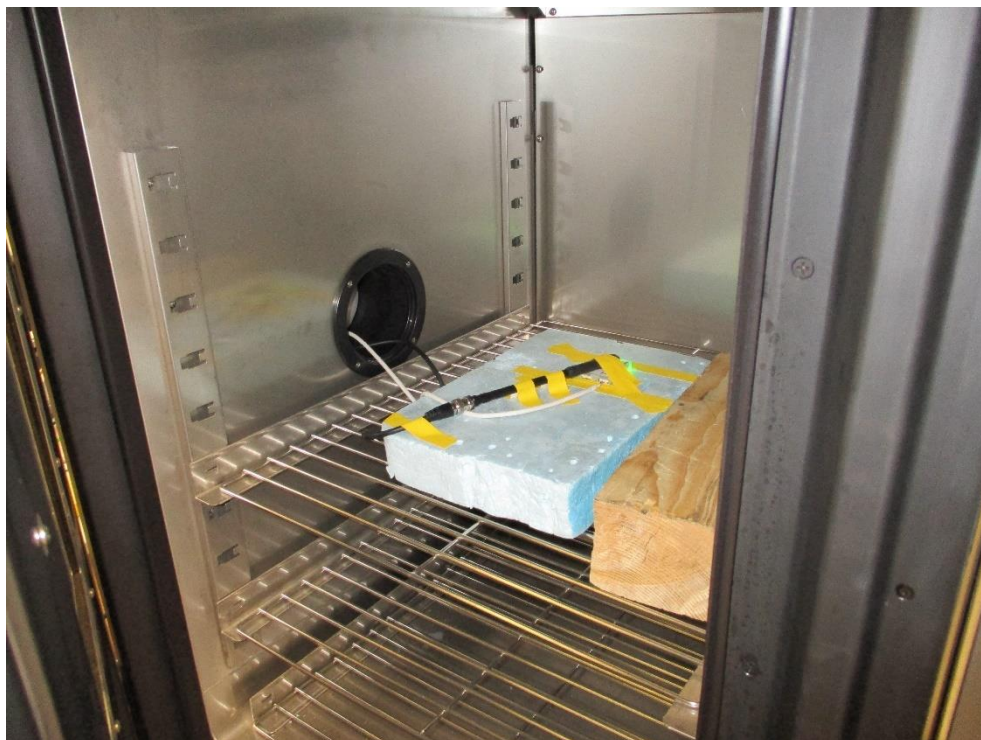
Figure 14 - Test setup for carrier frequency stability
