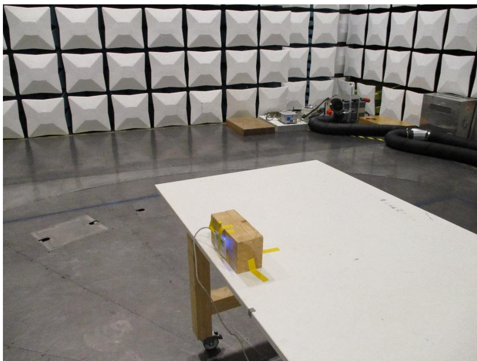
Figure 13 - Test setup for radiated emission 9kHz-30MHz
