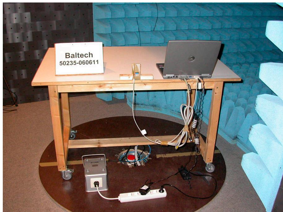
**Test setup for radiated emission measurement
