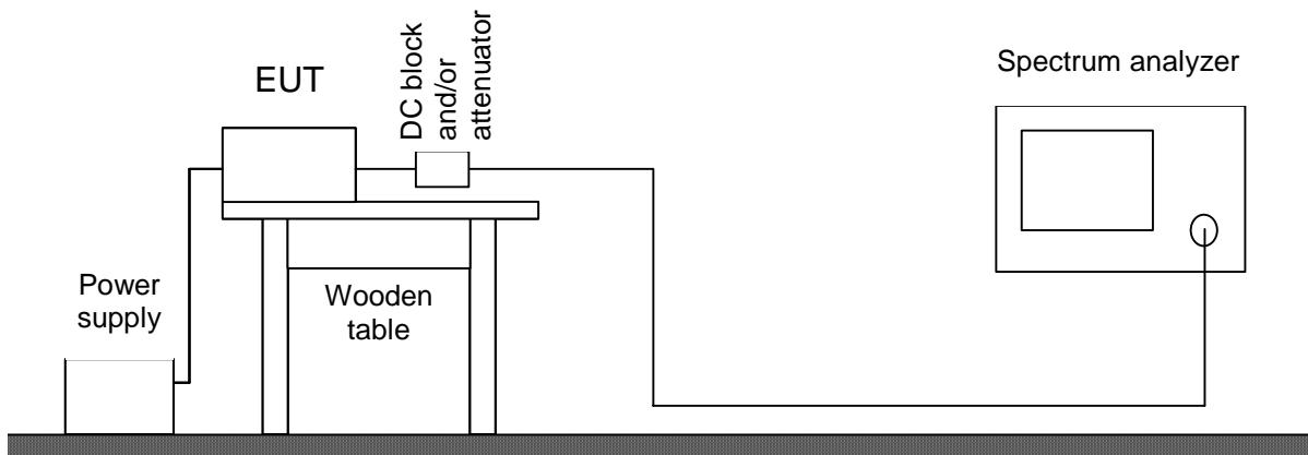
Test instruments used for conducted measurements:
