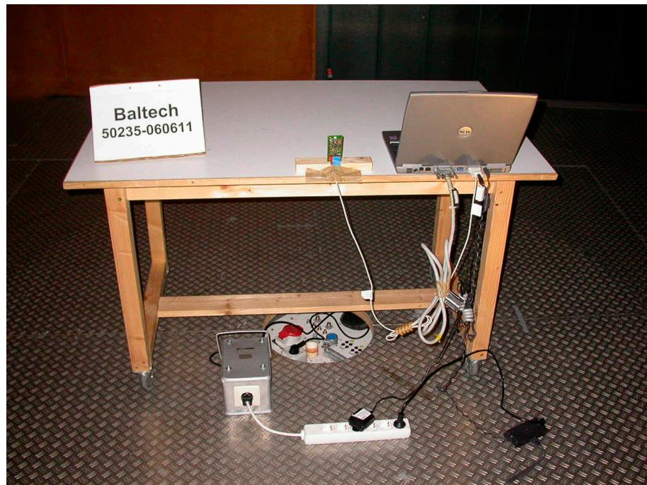
**Test setup for radiated emission measurement
