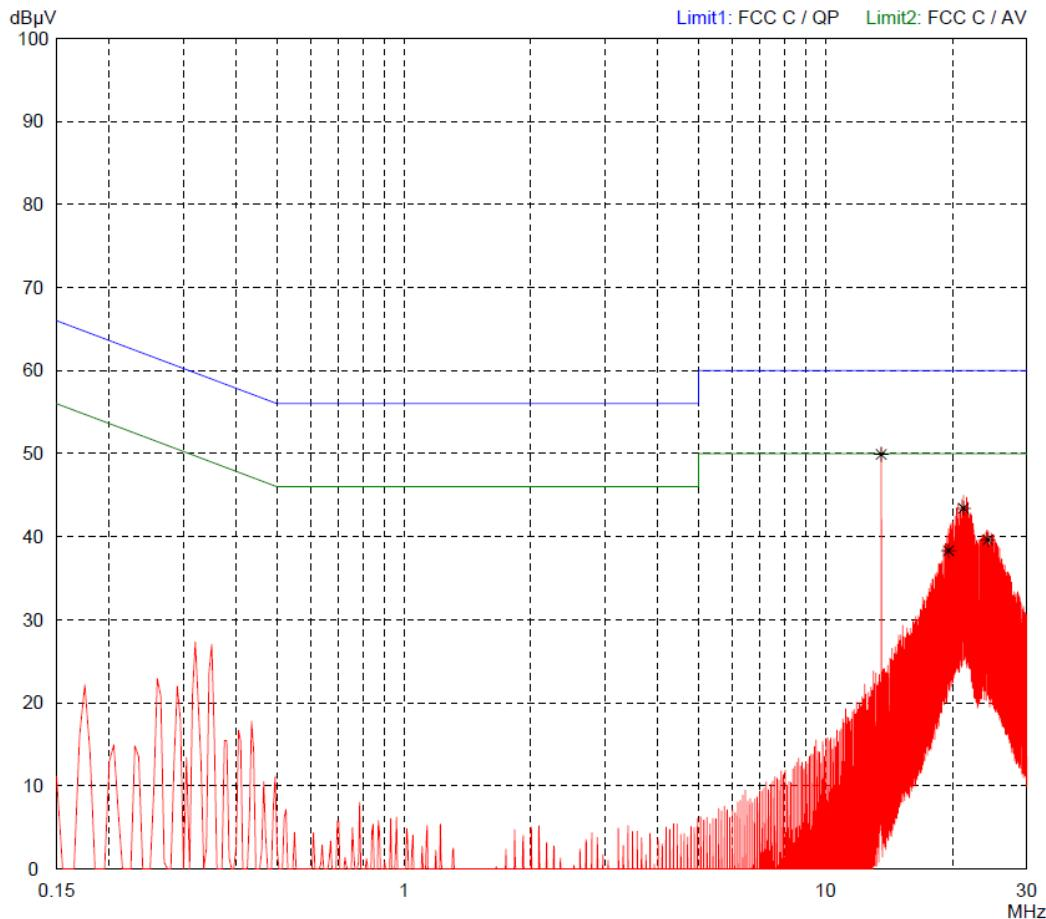
Conducted Emission Test 150 kHz - 30 MHz
