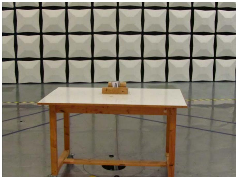
**Test setup for radiated emission measurement
