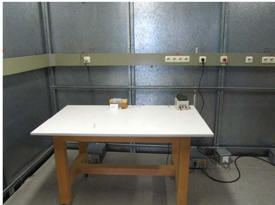
**Test setup for conducted AC powerline emission measurement**
