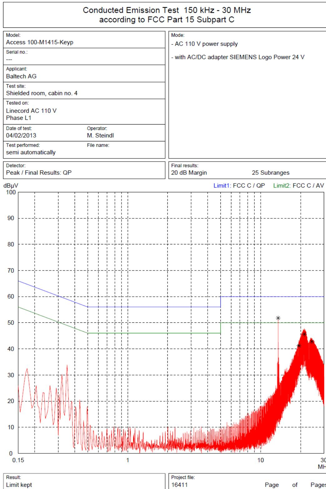
Conducted Emission Test 150 kHz - 30 MHz
